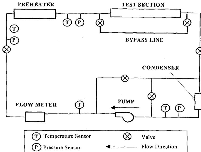
Figure 1: Test Section Schematic
