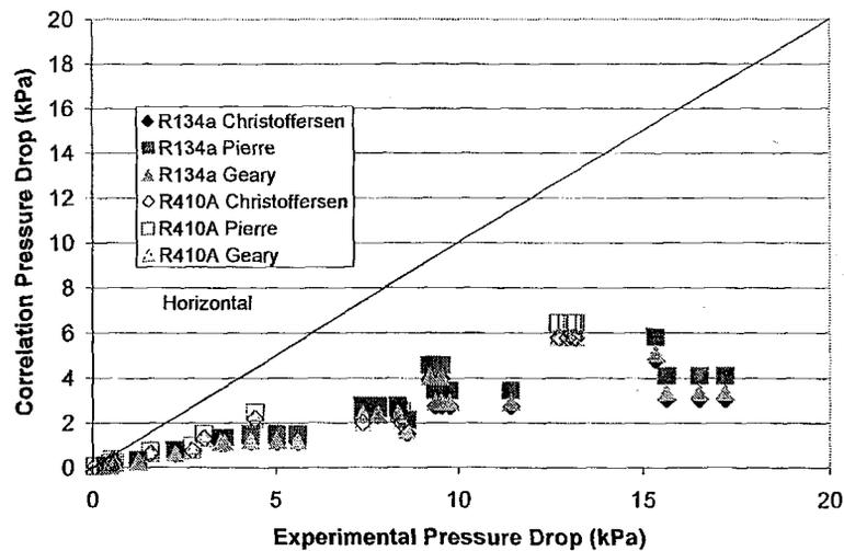
Figure 6: Comparison of Experimental and Correlation Test Section Pressure Drops
