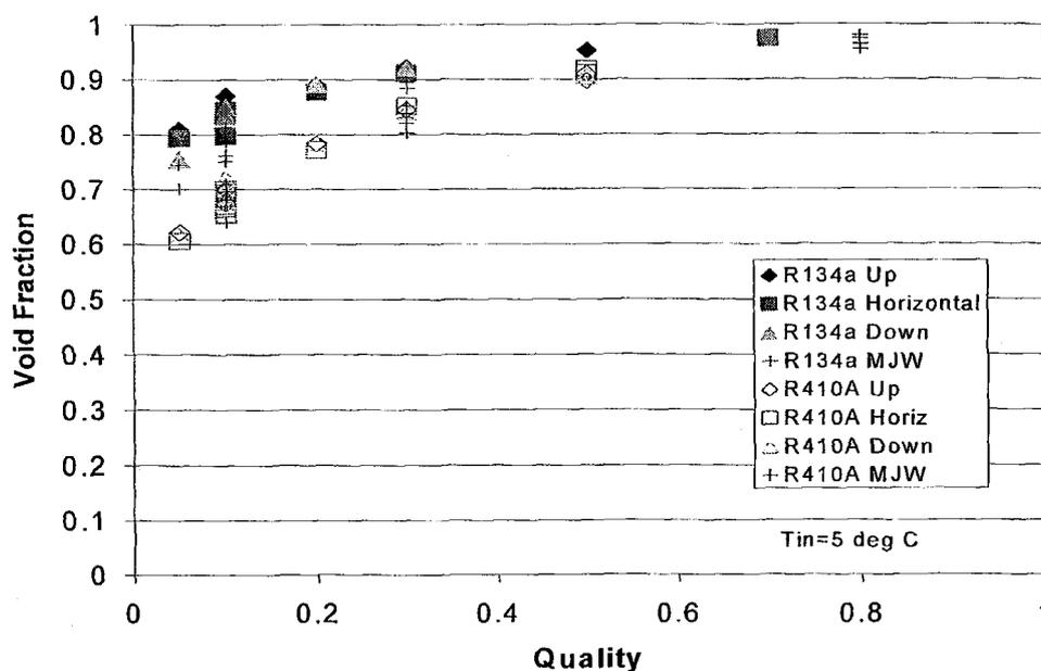
Figure 3: Return Bend Void Fraction Plot
