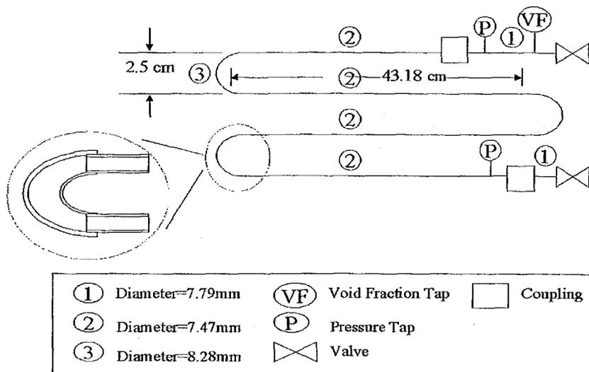
Figure 2: Return Bend Diagram
