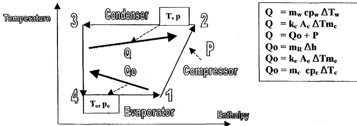
Figure 3: Simplified model of a refrigeration machine
