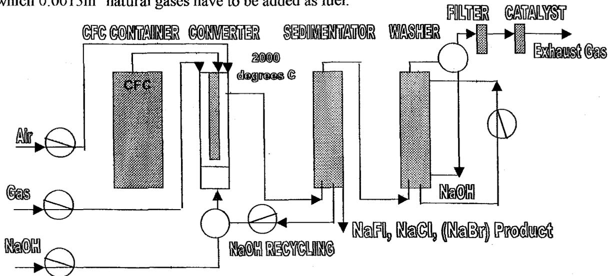
**Figure 2:** Process Chart of the Chemical Decomposer
