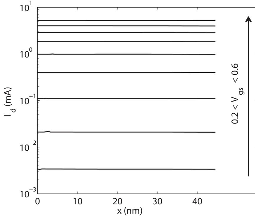
FIG. 11: Spatial current along the transport direction  $x$  of the Si GAA NW FET with a diameter  $d=2.5$  nm and in the presence of electron-phonon scattering. The currents are calculated at  $V_{ds}=0.6$  V and  $0.2 \leq V_{gs} \leq 0.6$  V.
