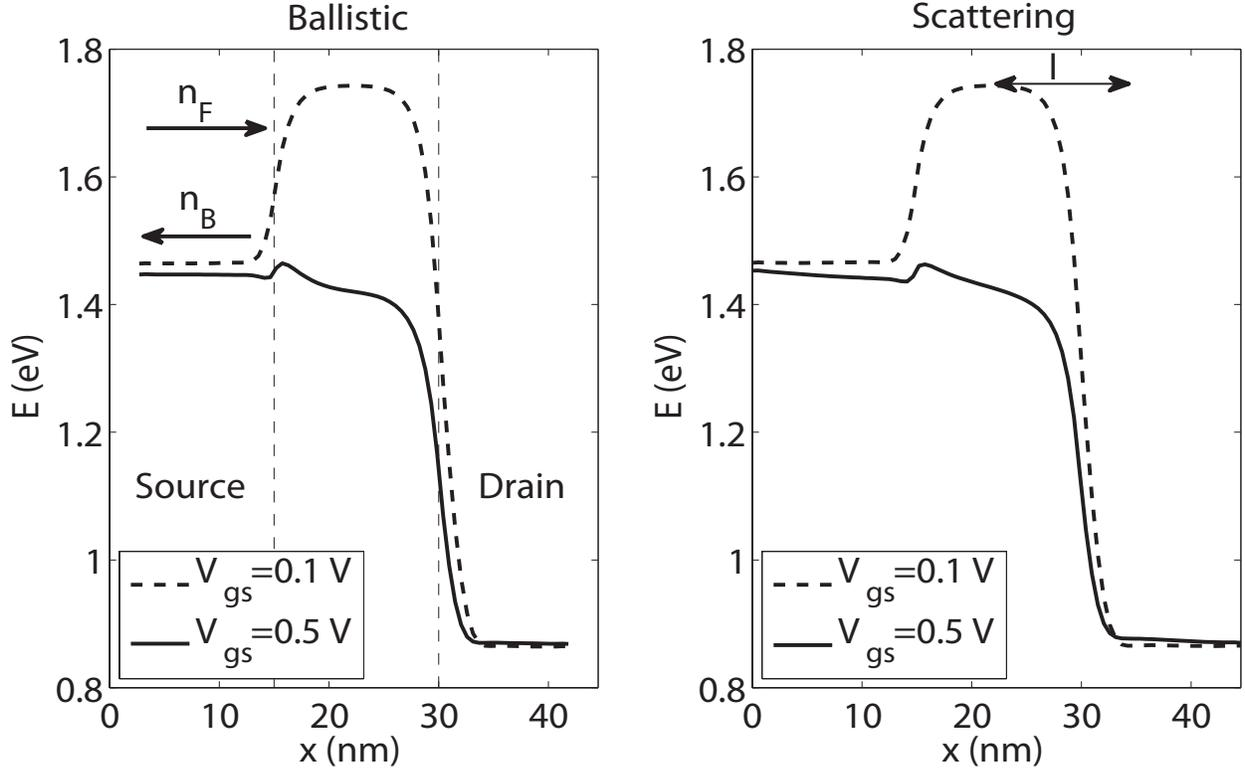
FIG. 8: Conduction band edges at  $V_{ds}=0.6$  V,  $V_{gs}=0.1$  V (dashed lines) and  $V_{gs}=0.5$  V (solid lines) in the nanowire with  $d=2.5$  nm. The band edges in case of ballistic transport are shown in the left subplot, those with electron-phonon scattering in the right subplot. The variable  $n_F$  ( $n_B$ ) describes the electrons moving forwards (backwards) to (from) the gate,  $l$  is the critical length for backscattering<sup>65</sup>.
