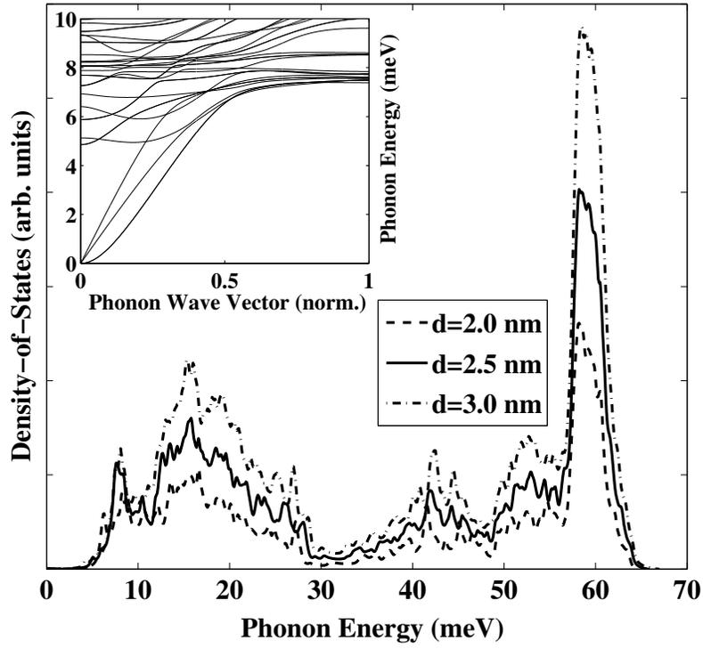
FIG. 2: Density-of-states of the confined phonons in a Si nanowire with a diameter  $d=2.0$  nm (dashed line),  $d=2.5$  nm (solid line), and  $d=3.0$  nm (dashed-dotted line). The inset shows the lowest part of the phonon bandstructure in the nanowire with  $d=2.5$  nm.
