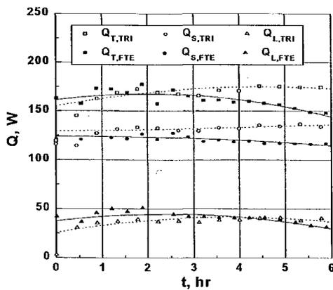
Fig.4 The heat transfer rate under frosting
