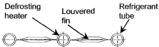
Figure 1. The shape of Tri-tube Sectional area
