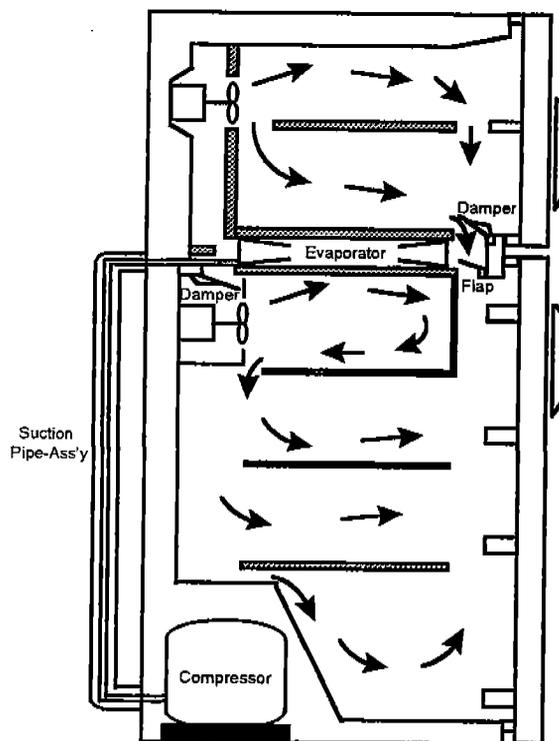
Figure 3. Schematic of the RF unit equipped with SEDS system
