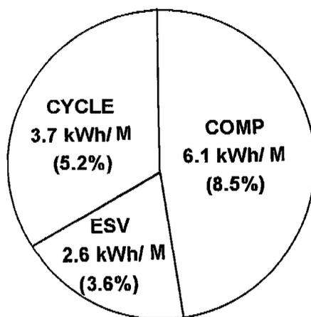
Figure 6. Contribution of the SEDS cycle for the reduction of energy consumption
