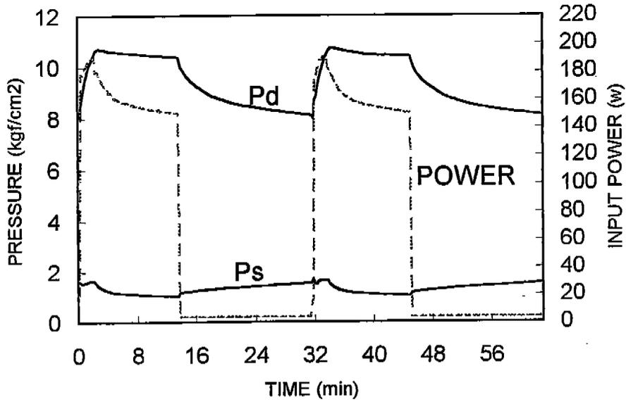
Figure 5. Pressure and power profiles for the SEDS system
