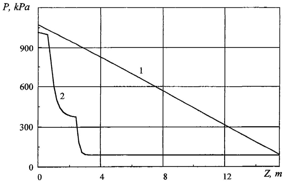
Fig. 1: Typical change of pressure at R134a flow in a long cooled capillary tube: 1- refrigerant pressure; 2 - vapor pressure corresponding to refrigerant temperature.
