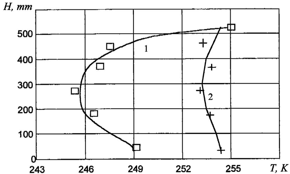
Fig. 2 : Temperature distribution along the height of freezing chamber: 1 - short capillary tube; 2 - long capillary tube ( $\square$ ,  $+$  - experimental data).
