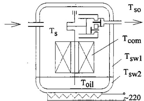
Fig. 1 Compressor shell model
