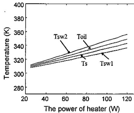
Fig. 2 Temperatures variation with power of oil heater
