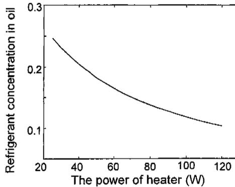
Fig. 3 Concentration of refrigerant variation with power of oil heater
