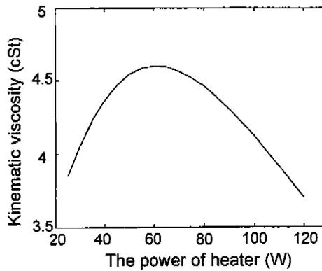
Fig. 4 Viscosity variation with power of oil heater
