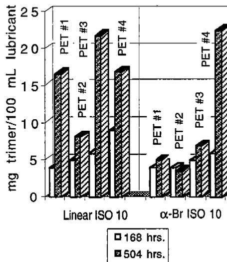
Figure 2. Extraction of PET Trimer From Several Slot Liner Materials by ISO 10 POEs (160 °C, 1 and 3 wks.)
