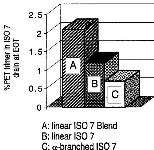
Figure 5. Effect of ISO 7 POE Structure on PET Trimer Extraction.
