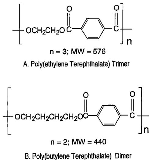
**Figure 1. Low Molecular Weight Oligomers Extracted from PET and PBT**
