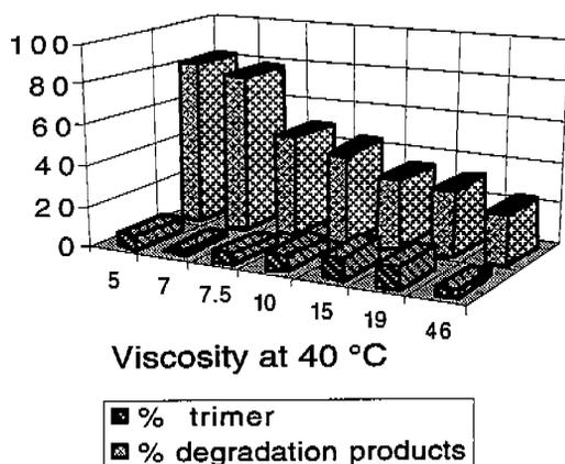
**Figure 3. Effect of POE Viscosity on Extraction of Low Molecular Weight PET Components.**
