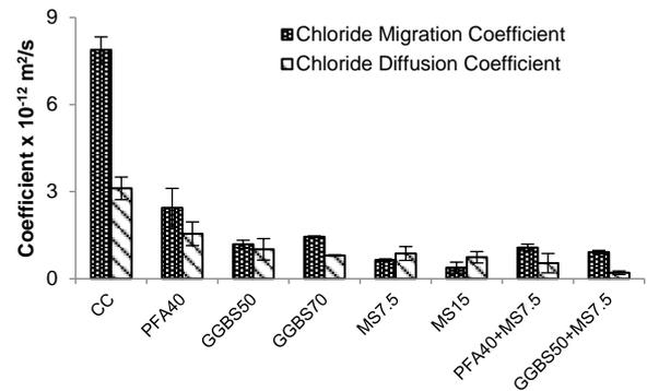
**Fig. 7.** Chloride transport coefficients for various mixes
