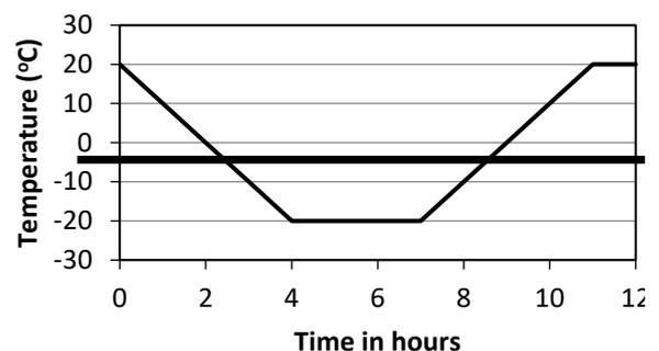
Fig. 2. Freeze-thaw cycle used for salt-scaling test
