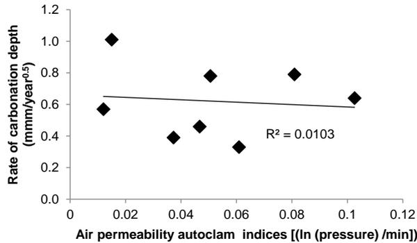
**Fig. 12.** Air permeability indices and carbonation depth relationship
