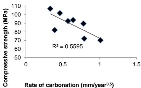
**Fig. 13.** Compressive strength and rate of carbonation relationship
