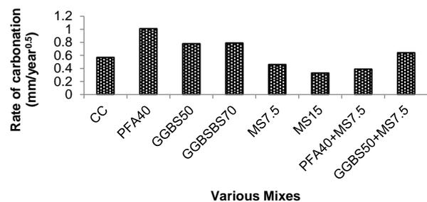
**Fig. 11.** Rate of carbonation for various mixes
