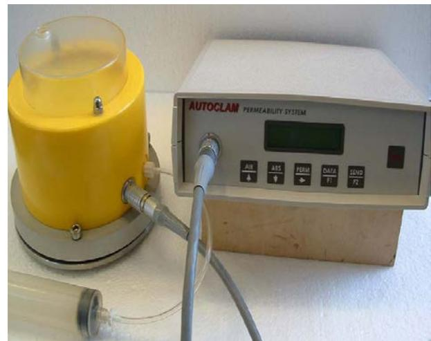
**Fig. 1.** Autoclam permeability apparatus
