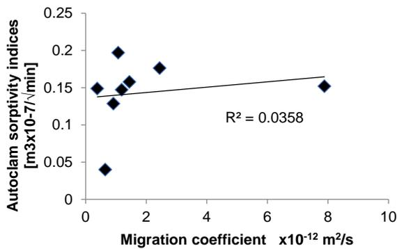
**Fig. 9.** Sorptivity indices and chloride migration coefficients relationship
