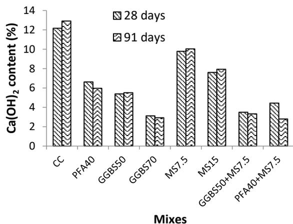
**Fig 3.**  $\text{Ca(OH)}_2$  contents for various mixes
