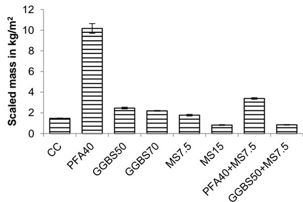
**Fig. 14.** Scaled mass of concrete after 400 cycles
