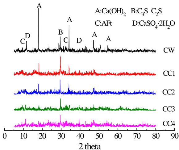
**Fig. 13.** XRD curves of the specimens in water and sewage
