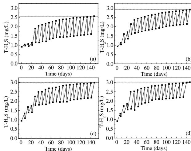
**Fig. 4.** Evolution diagrams of T-H<sub>2</sub>S values of sewage with different concentration: a) SC1; b) SC2; c) SC3; d) SC4
