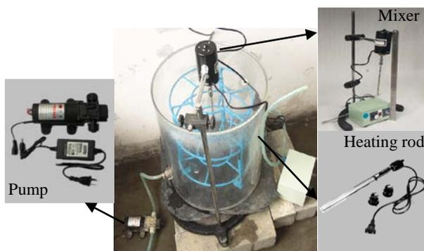
**Fig. 1.** In-house simulation chamber for sewage corrosion test
