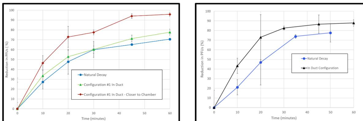
**Figure 3.** *Left.* MS2 challenge data for an in-duct gas-phase H<sub>2</sub>O<sub>2</sub> generator at 101 CFM 6 ACH, 1007 ft<sup>3</sup> chamber. *Right.* MS2 challenge data for an in-duct gas-phase H<sub>2</sub>O<sub>2</sub> generator at 336 CFM, 20 ACH, 1007 ft<sup>3</sup> chamber
