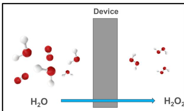
**Figure 1.** Schematic of the gas-phase  $\text{H}_2\text{O}_2$  generator showing the utilization of atmospheric water and conversion into  $\text{H}_2\text{O}_2$  via the photocatalytic oxidation process.
