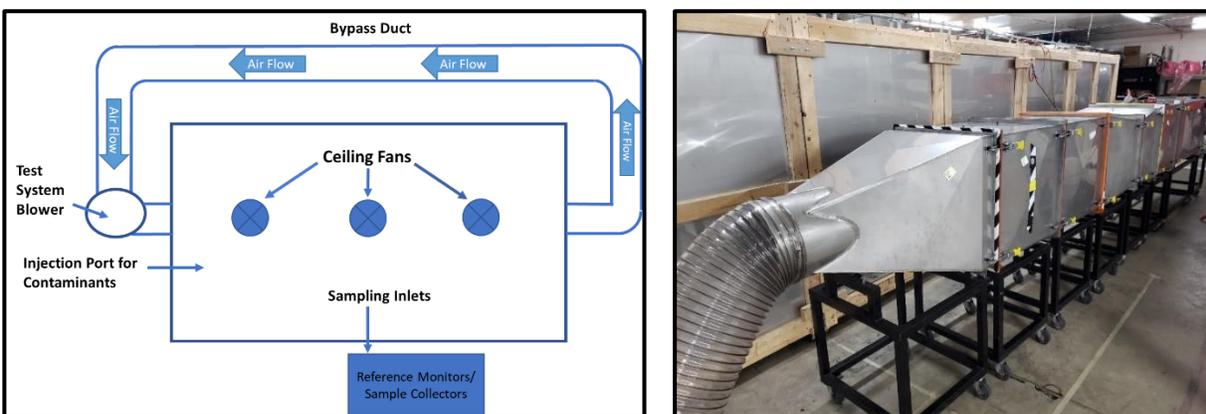
**Figure 2.** *Left.* Environmental test chamber schematic depicting placement of various sensors, injection location, and sampling. *Right.* Image of the chamber with the bypass recirculating duct.
