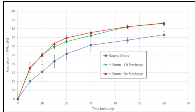
**Figure 4.** MS2 challenge data for an in-room  $H_2O_2$  generator at 410 CFM, 6 ACH, 4096 ft<sup>3</sup> chamber.
