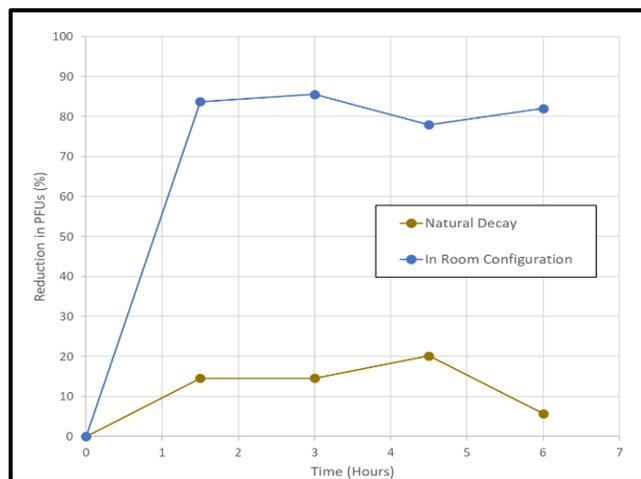
**Figure 5.** Surface MS2 deactivation data for an in-room  $H_2O_2$  generator.
