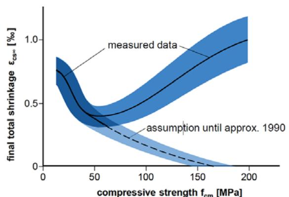
**Fig. 3.** Final Shrinkage of Concrete (Source Moser-Pfeifer, Weimar University as presented by H.S. Muller, TG10.1 Barcelona 2017)
