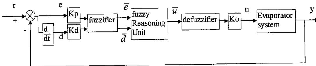
Fig. 2 The block diagram of a fuzzy control system
