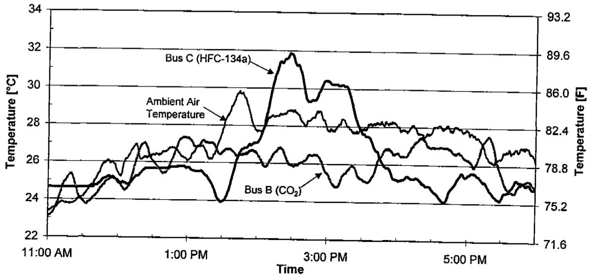
**Fig. 4: Variation of the Interior Air Temperature of Bus B (Carbon Dioxide A/C System) and Bus C (Standard HFC-134a A/C System). Bad Hersfeld, August 05, 1997.**
