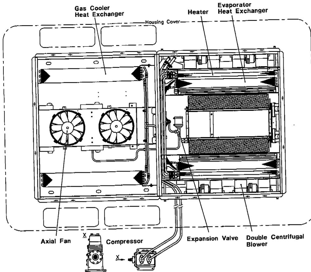
Fig.2: Plan View without housing cover of the Prototype Roof-Mount Bus A/C Unit
