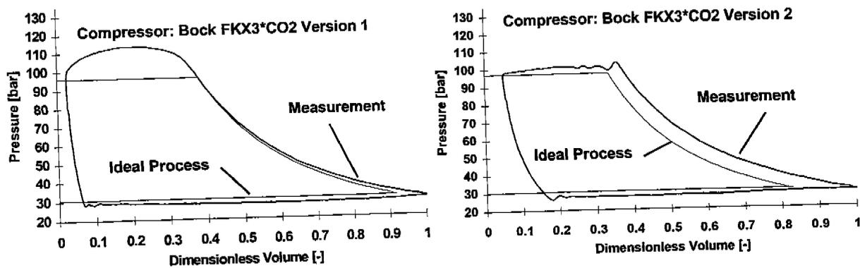
Fig. 7: Measured Indicator Diagrams.
