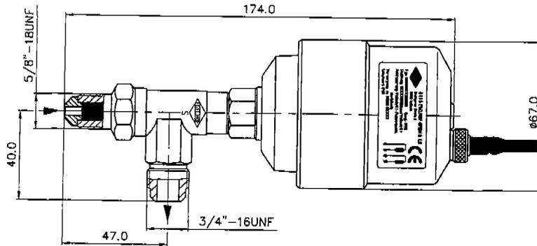
**Fig. 3: Electronic Expansion Valve**
