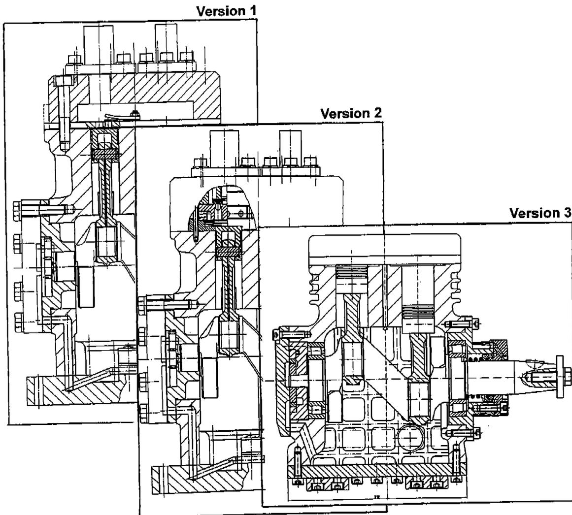
Fig. 6: Design Steps of Bock CO<sub>2</sub>-Compressor.
