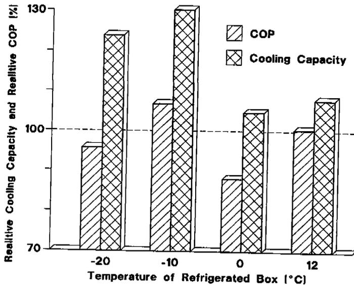
**Fig. 5: Relative COP and Relative Cooling Capacity of the CO<sub>2</sub>-System with Internal Heat Exchanger (Ambient Air Temperature  $t_{amb}=30\text{ }^{\circ}\text{C}$  (86F), 100%=Cooling Capacity of System without Internal Heat Exchanger)**
