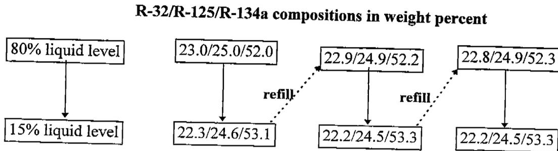
The maximum change in composition is 1.3% R-134a at 15% liquid level, and the composition stabilizes after the second refilling of the OEM storage tank. The compositions are within the specifications of 21-25% for R32, 23 - 27% for R-125, and 50 - 54% for R-134a. But there are several situations that could cause the compositions to go outside specifications.
