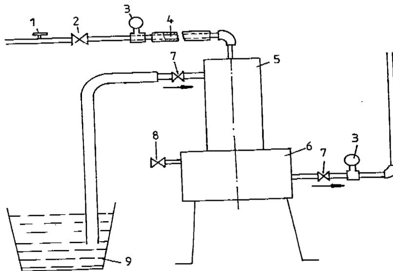
**Fig 2. Steam Operated Water Pump Test Stand**
