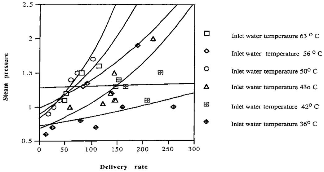
Fig. 4. Water deliverly vs steam pressure
