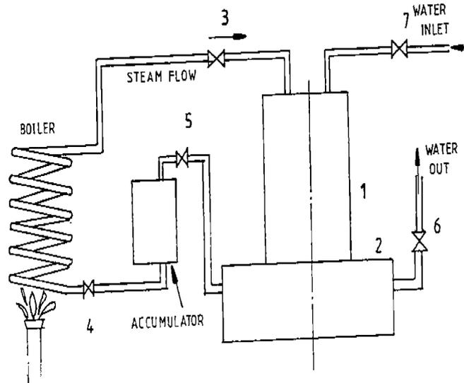
**Fig 1 Steam operated water pump**
