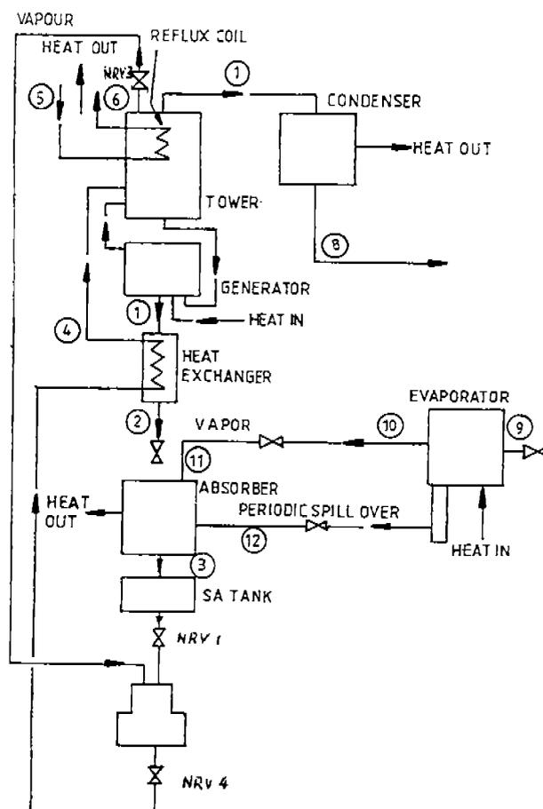
**Fig 6. Ammonia - Water Single Stage Absorption Refrigeration System with Multi phase thermal Pump**
