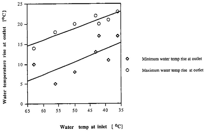
Fig. 5 Water temp at inlet vs water rise at outlet.
