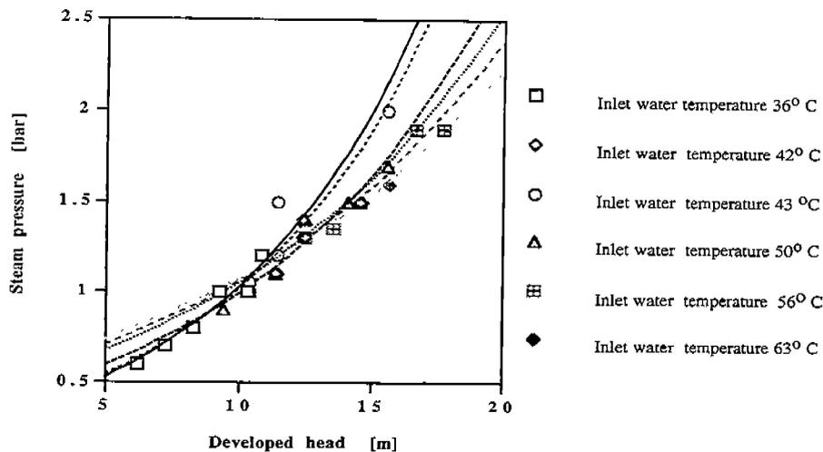
Fig. 3. Developed head Vs steam gauge pressure.
