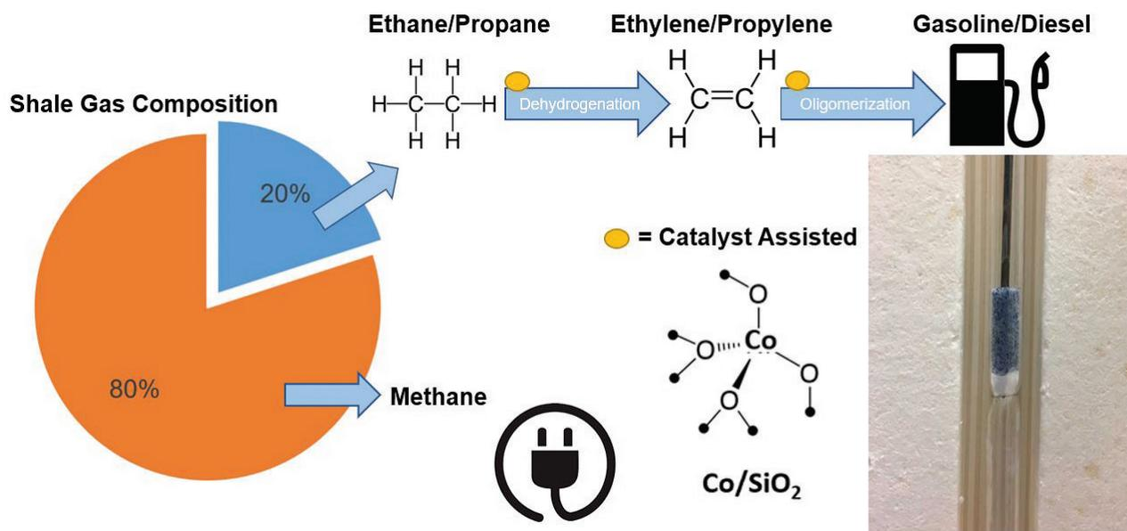
The process of transforming excess ethane and propane from shale gas is shown as a two-step process. Dehydrogenation processes ethane and propane into ethylene and propylene, which are further processed into transportation fuels in oligomerization. Both reactions are catalyzed by a Co<sup>2+</sup>/SiO<sub>2</sub> catalyst.
