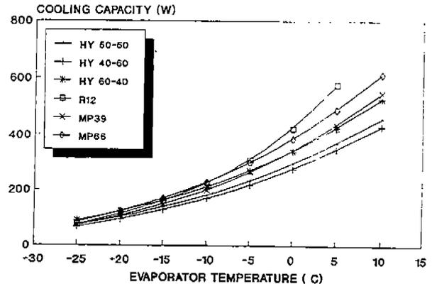
Fig 4 COMPARISON OF COOLING CAPACITY OF HYDROCARBON MIXTURES FOR REFRIGERATOR (CONDENSER TEMP = 55 C)
