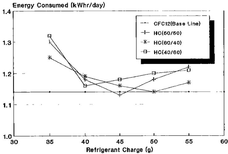
Fig.7 ENERGY CONSUMPTION VS CHARGE
