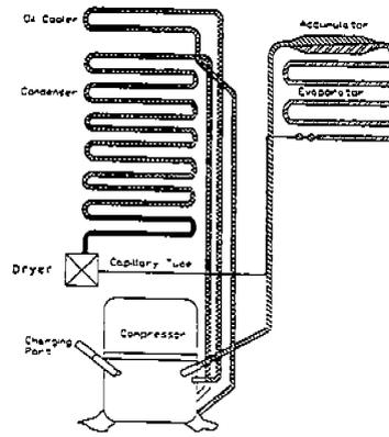
Fig.2 Schematic Diagram of Refrigerator
