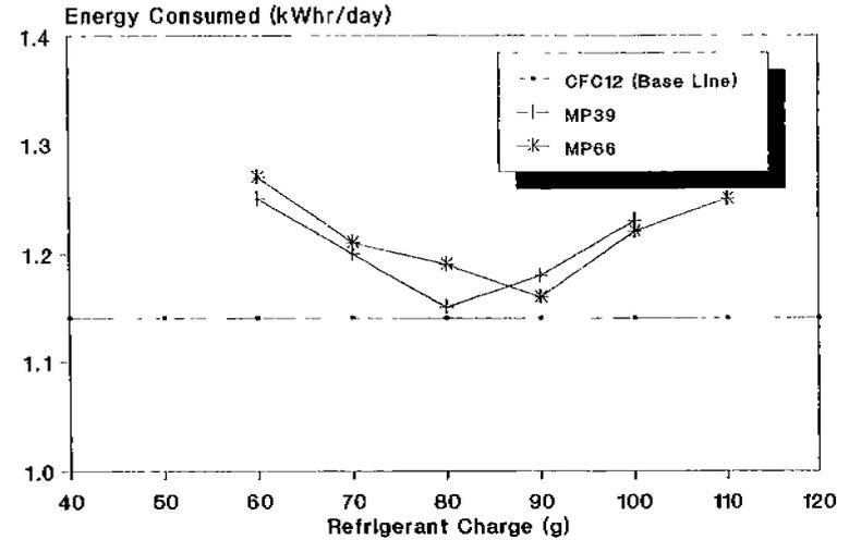
Fig.8 ENERGY CONSUMPTION VS CHARGE
