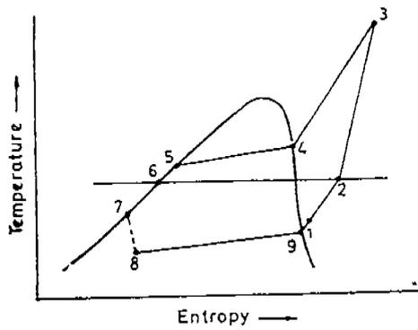
Fig.3 T-S diagram of refrigerator
