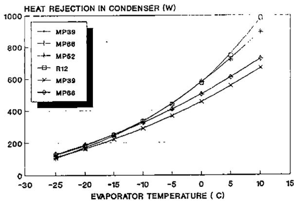
Fig 5 COMPARISON OF HEAT REJECTION IN CONDENSER OF TERNARY MIXTURES FOR REFRIGERATOR (CONDENSER TEMP = 55 C)
