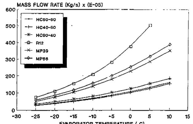
Fig 6 COMPARISON OF MASS FLOW RATE FOR HYDROCARBON MIXTURES IN REFRIGERATOR (CONDENSER TEMP = 55 C)
