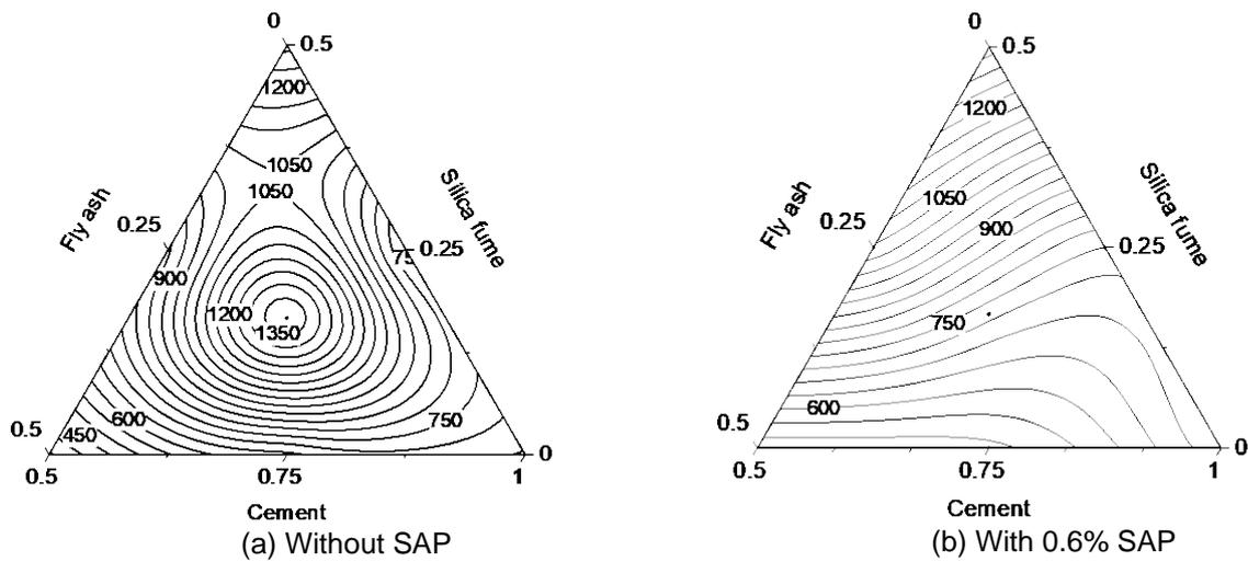
Fig. 6. Total shrinkage of UHSC at 3d
