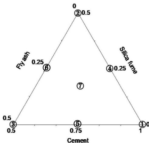
**Fig. 2.** Ternary cementitious materials according to simplex-centroid design
