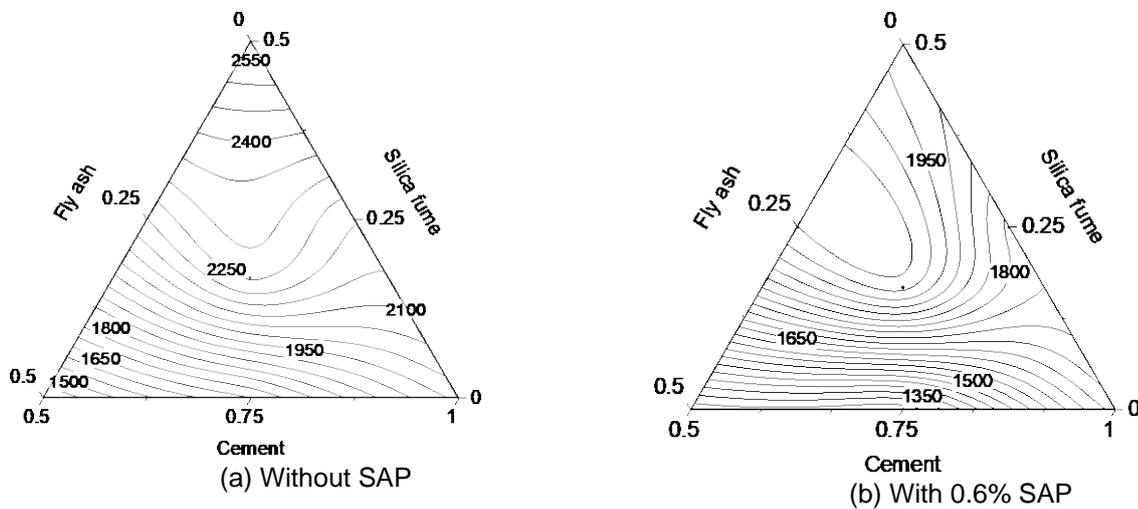
Fig. 7. Total shrinkage of UHSC at 28d
