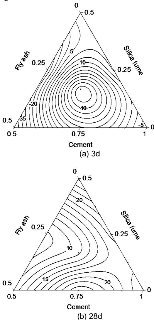
**Fig. 8.** Effectiveness of internal curing at different ages
