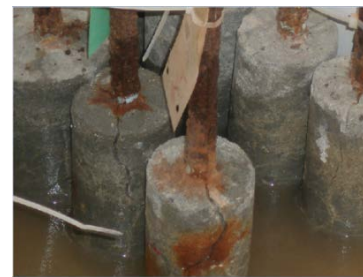
Fig. 1. Test specimens: a) schematic diagram of typical test-specimen; b) typical corrosion state
