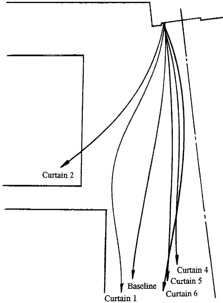
**Figure 3 - Projected paths of air curtain peak velocities**
