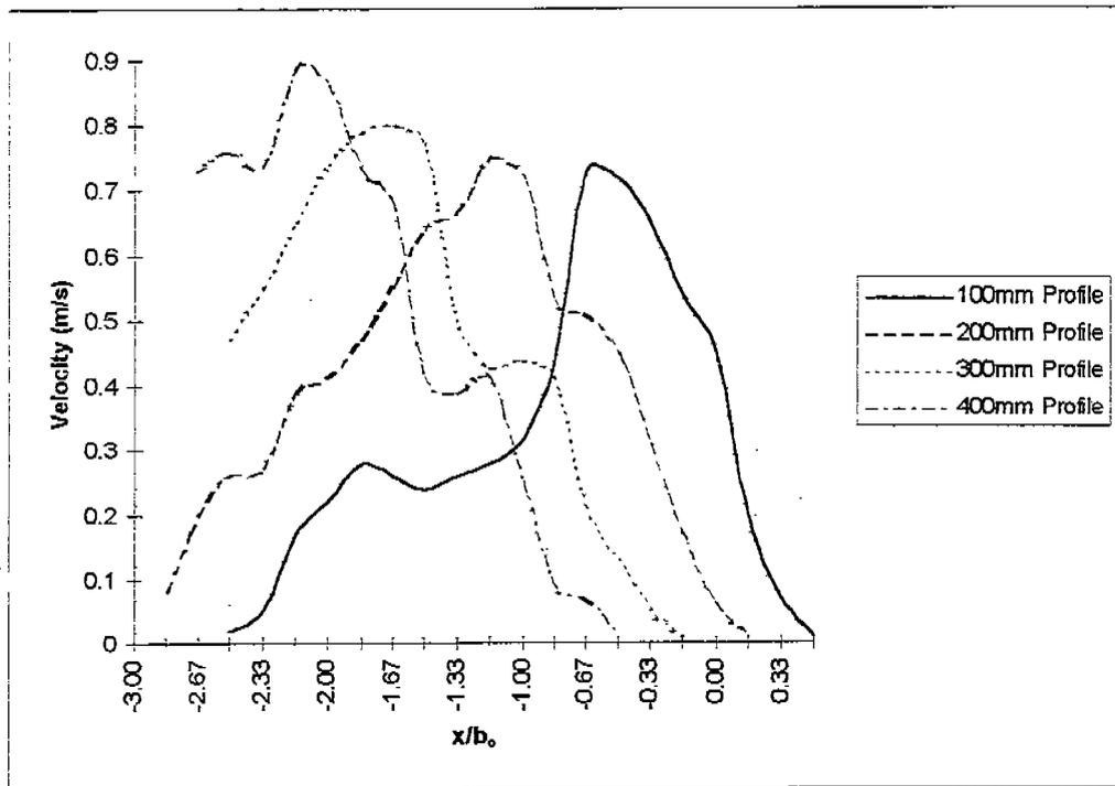
Figure 2 - Velocity profiles taken for baseline case 610mm from left hand end of unit
