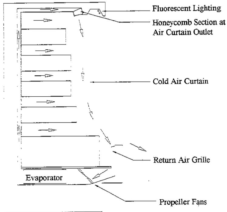
Figure 1 - Typical operation of refrigerated multideck case
