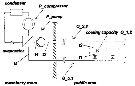
Figure 2: Secondary Refrigerant System
