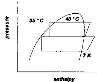
Figure 4: Process of the two Stage Ammonia Cycle
