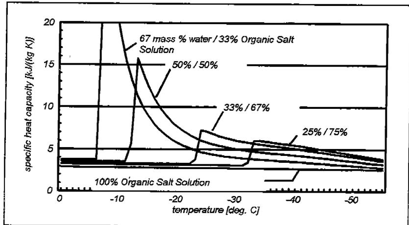
**Figure 7:** Ice Slurry as secondary refrigerant
