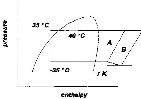
Figure 3: Process of the Direct Evaporation Cycle
