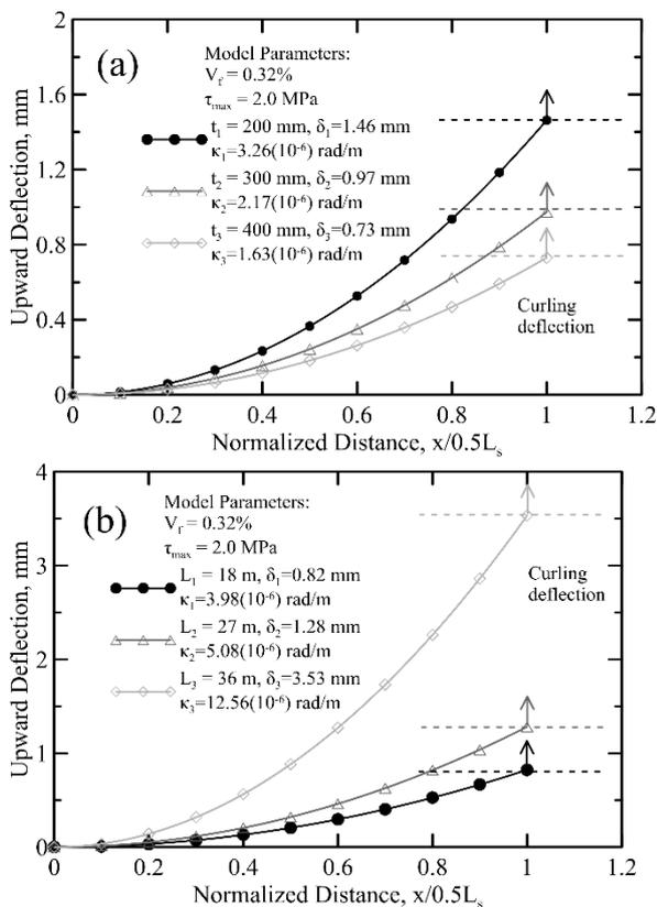
**Fig. 13.** Tip curling deflection increase at the cracked section with effect of slab thickness, and b) effect of slab length (Destrée et al., 2015).
