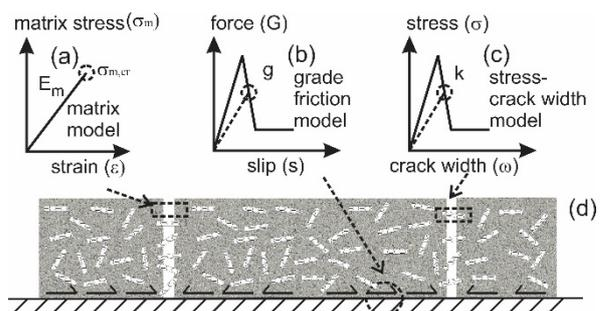
**Fig. 10.** Mechanical behavior of cracked FRC slab: a) matrix strength for cracking criterion, b) nonlinear spring model simulating the frictional force, c) stress-crack width model, d) cracked cement composite (Destree et al., 2015).
