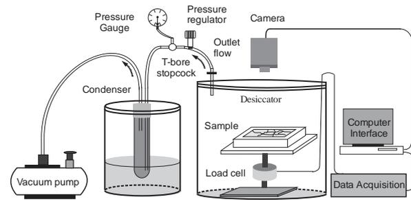
Fig. 1. Schematic of vacuum drying test setup
