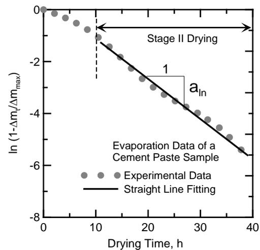
Fig. 2. (a) Experimental moisture loss and its Simulation for cement paste (b) Derivation of model coefficients for linearized curve of moisture loss  $\ln(1 - \Delta M_t / \Delta M_{\max})$  vs. time in stage II.
