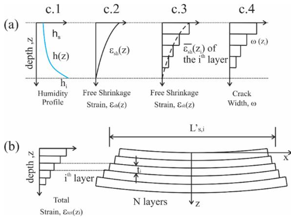
**Fig. 11.** Modelling procedure for curling of a slab. a) Slab strain distribution discretized into  $N$  layers and the imposed strain gradient due to humidity profile. b) Distribution of total strain into the curvature and tip deflection (Destrée *et al.*, 2015).
