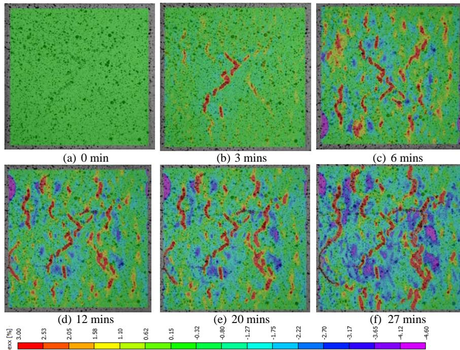
**Fig. 3:** Sequential growth of shrinkage cracks observed in an alkali activated slag specimen within the first hour of the test (Dey *et al.*, 2015).
