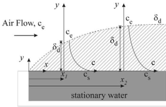
**Fig. 6.** Distribution of water vapor concentration and diffusion boundary layer thickness in laminar, and turbulent regions near concrete interface
