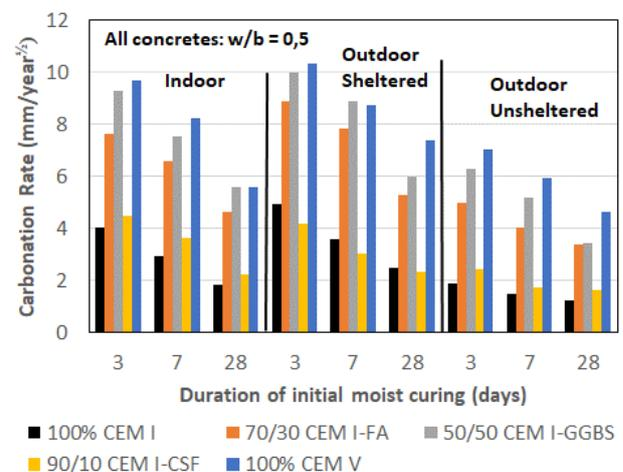
**Fig. 7.** Effects of micro-climate variations on the rate of carbonation of concretes made with a range of binder types (Alhassan, 2014)
