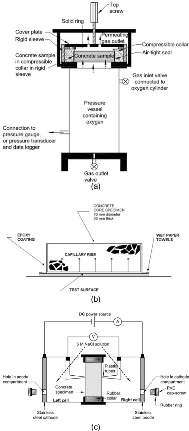
**Fig. 2.** Three South African durability index tests: (a) falling-head oxygen permeability test; (b) water sorptivity test and (c) chloride conductivity test.
