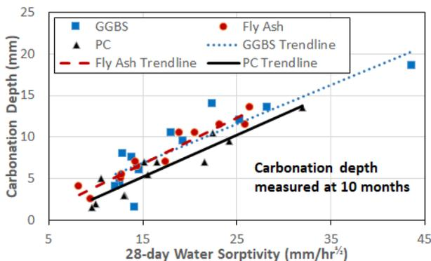
**Fig. 4.** Correlation between water sorptivity as a durability index and 10-month natural carbonation (Ballim, 1996)
