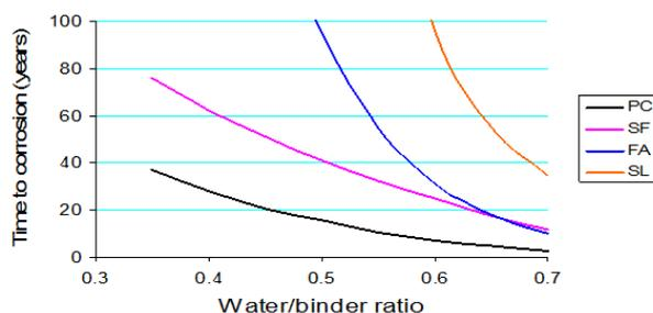
**Fig. 9.** An example of the use of the chloride conductivity index to predict the time to initiation of corrosion in reinforced concrete with different binder types
