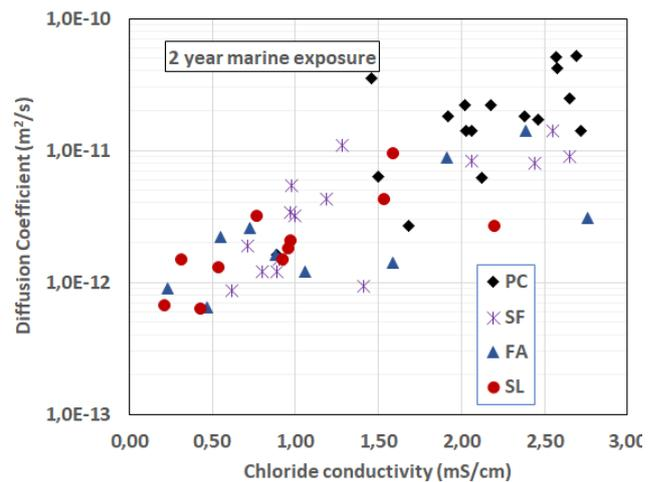
**Fig. 6.** Correlation between chloride conductivity test results and the measured chloride diffusion coefficient for concretes exposed in a marine environment (adapted from Alexander *et al.*, 1999)
