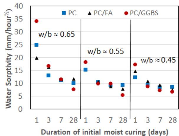
**Fig. 3.** Sensitivity of the water sorptivity index to variations in initial curing duration, binder type and w/b ratio in concrete (adapted from Ballim, 1993a)
