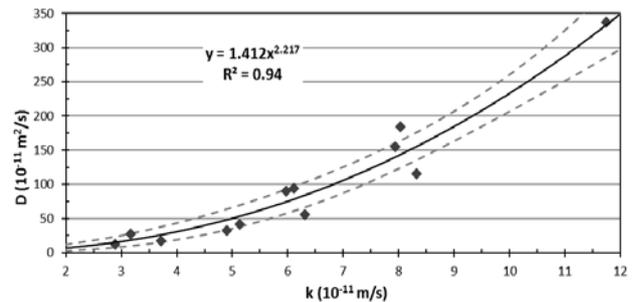
**Fig. 5.** Permeability (k) vs. effective dry diffusion coefficient (with line of best fit and 95% confidence intervals), range of concretes with various binders (Salvoldi *et al.*, 2015)
