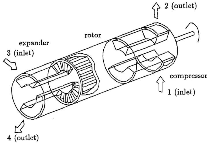
Figure 5: Sketch of a pressure wave machine.
