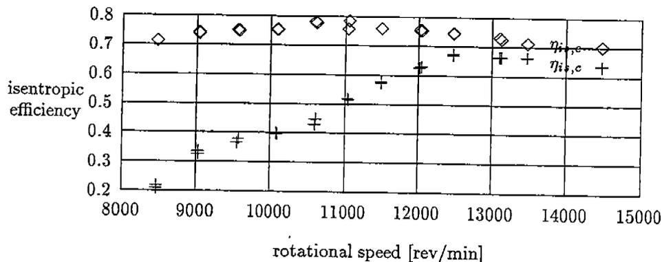
Figure 7: Measured efficiencies for the pressure wave machine.
