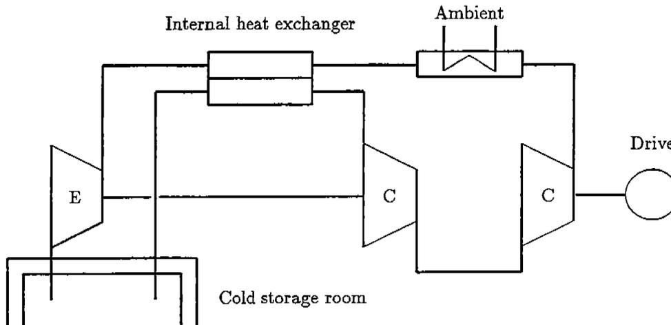
Figure 2: Bootstrap open cycle configuration with internal heat exchanger.
