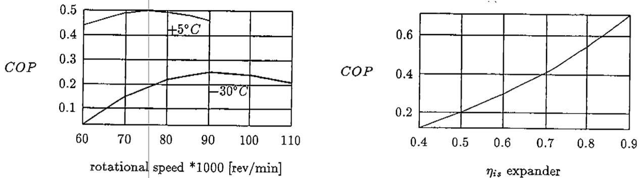
Figure 4: Left: Simulated  $COP$  results for  $+5^{\circ}C$  and  $-30^{\circ}C$  in the cold storage room. Right: Simulated  $COP$  results as a function of the efficiency of the expander.
