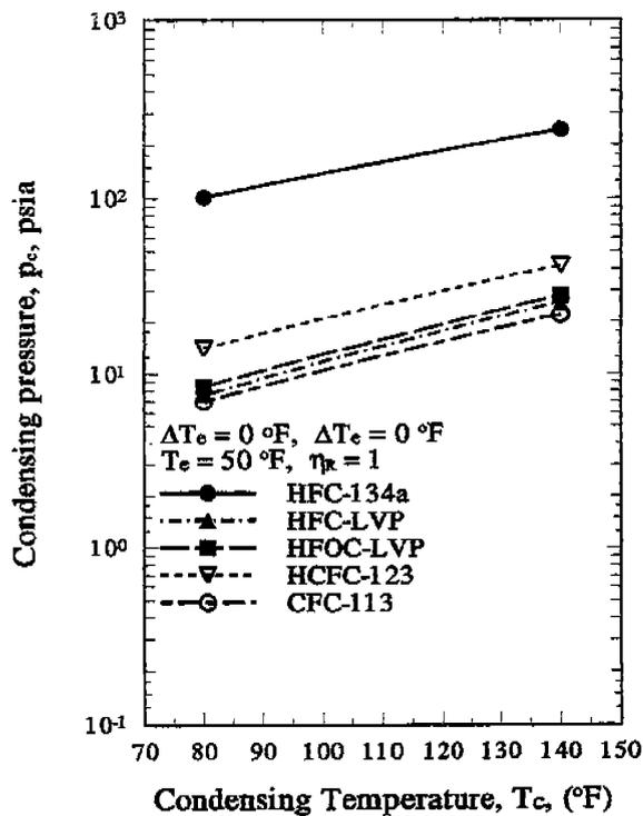
Fig. 4 Condensing pressure  $p_c$  at various  $T_c$
