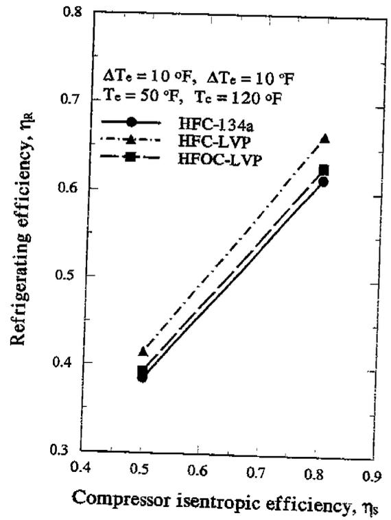
Fig. 6 Refrigerating efficiency  $\eta_R$  vs  $\eta_s$
