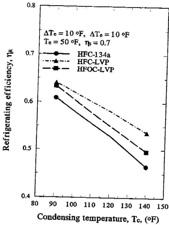
Fig. 7 Refrigerating efficiency  $\eta_R$  vs  $T_c$
