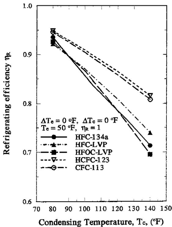
Fig. 1 Refrigerating efficiency  $\eta_R$  at various  $T_c$
