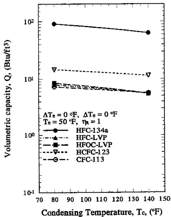
Fig. 3 Volumetric capacity  $Q$  at various  $T_c$
