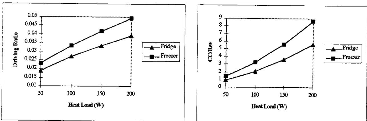
Figure 7. (a) Variation of the driving ratio with heat load for a thermoacoustic refrigerator and freezer, and (b) The CC rating of a vapour compression refrigerator and freezer at different heat loads.
