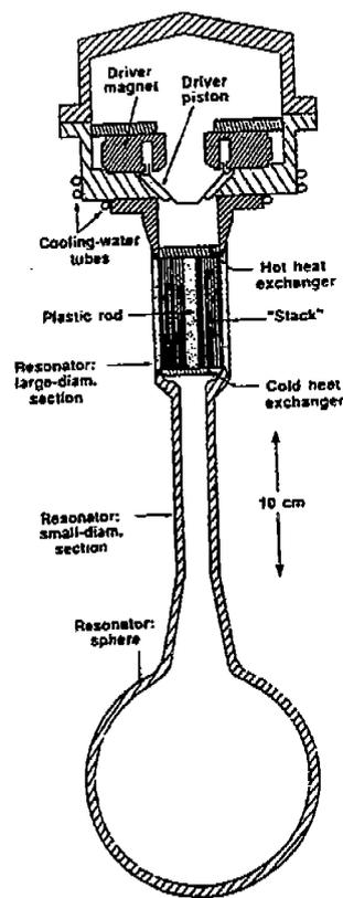
Figure 3. Hofler design thermoacoustic refrigerator
