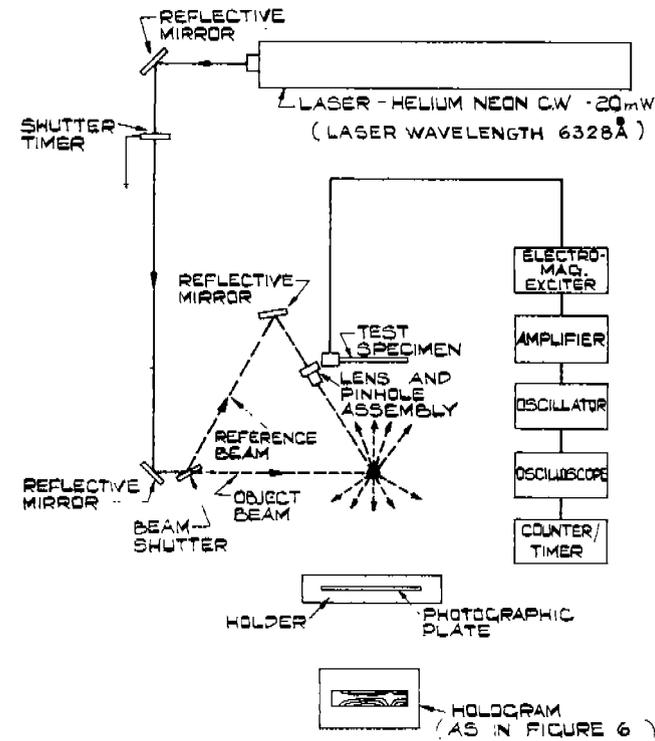
FIG 14 LAYOUT OF APPARATUS FOR HOLOGRAPHIC INTERFEROMETER
