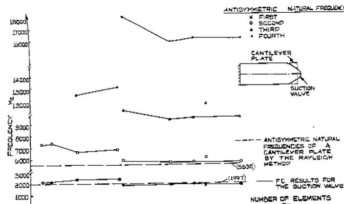
FIG 7(b) CONVERGENCE AND COMPARISON OF THE PREDICTED ANTISYMMETRIC NATURAL FREQUENCIES OF SUCTION VALVE REED WITH THE ANTISYMMETRIC NATURAL FREQUENCIES OF A TYPICAL CANTILEVER PLATE
