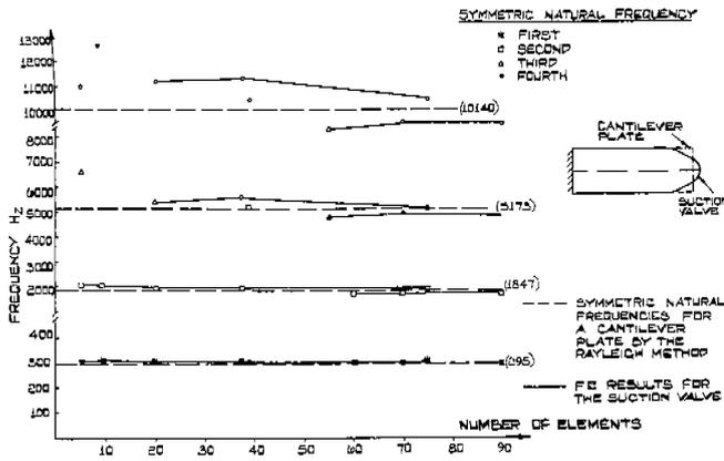
FIG 7(a) CONVERGENCE AND COMPARISON OF THE PREDICTED SYMMETRIC NATURAL FREQUENCIES OF SUCTION VALVE REED WITH THE SYMMETRIC NATURAL FREQUENCIES OF CORRESPONDING RECTANGULAR CANTILEVER PLATE
