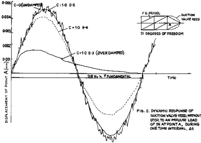
FIG. 8. DYNAMIC RESPONSE OF SUCTION VALVE REED, WITHOUT STOP, TO AN IMPULSE LOAD OF IN AT POINT A, DURING ONE TIME INTERVAL,  $\Delta t$
