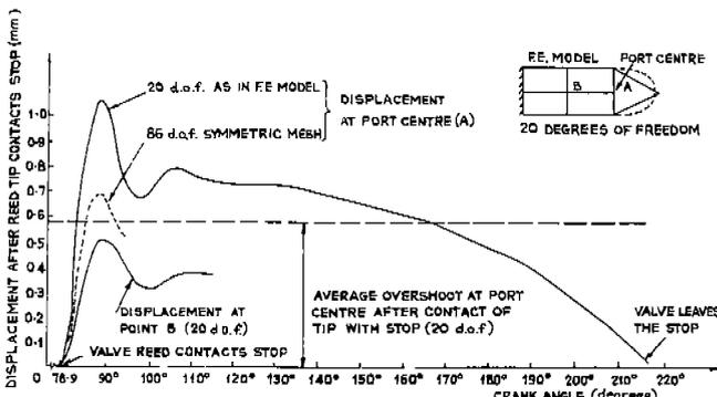
FIG. 9. SUCTION VALVE REED DISPLACEMENT AT THE CENTRE OF THE PORT AND AT POINT B AFTER THE VALVE REED TIP IS IN CONTACT WITH POINT STOP.
