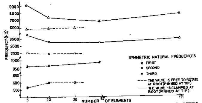
FIG 7(c) EFFECT OF DEGREE OF CLAMPING & CONVERGENCE OF THE PREDICTED SYMMETRIC NATURAL FREQUENCIES OF THE SUCTION VALVE WITH STOP AT TIP
