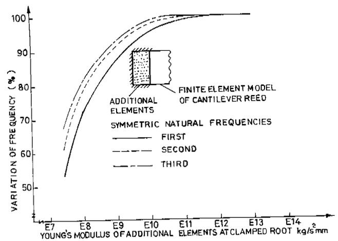
FIG 7(d) VARIATION OF SYMMETRIC NATURAL FREQUENCIES OF THE SUCTION VALVE REED WITH DEGREE OF ROOT CLAMPING
