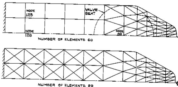
FIG 4 FINITE ELEMENT MODEL FOR HALF OF SUCTION VALVE REED WITH 135 DEGREES OF FREEDOM
