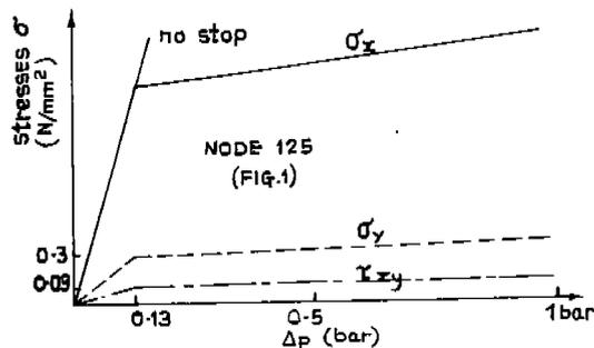
FIG. 4 EFFECT OF POINT STOP ON STATIC DISPLACEMENT AND STRESSES FOR CANTILEVER SUCTION VALVE REED
