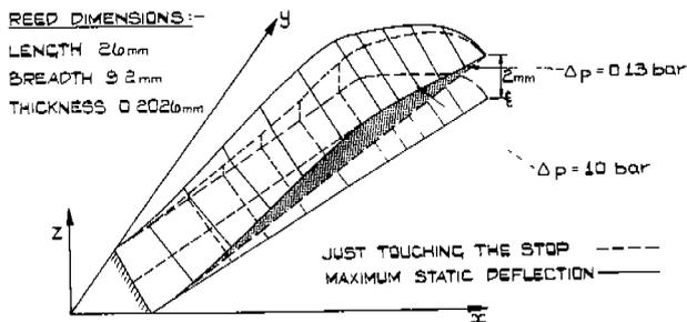
FIG. 2. STATIC DEFORMATION OF HALF SUCTION VALVE REED
