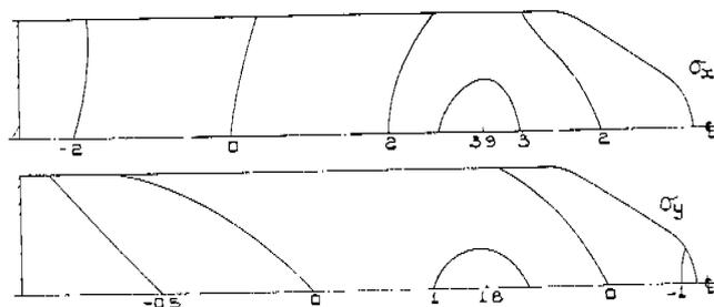
FIG.13 MAXIMUM STRESS  $N/mm^2$  FOR SUCTION VALVE REED DURING DYNAMIC OPERATION
