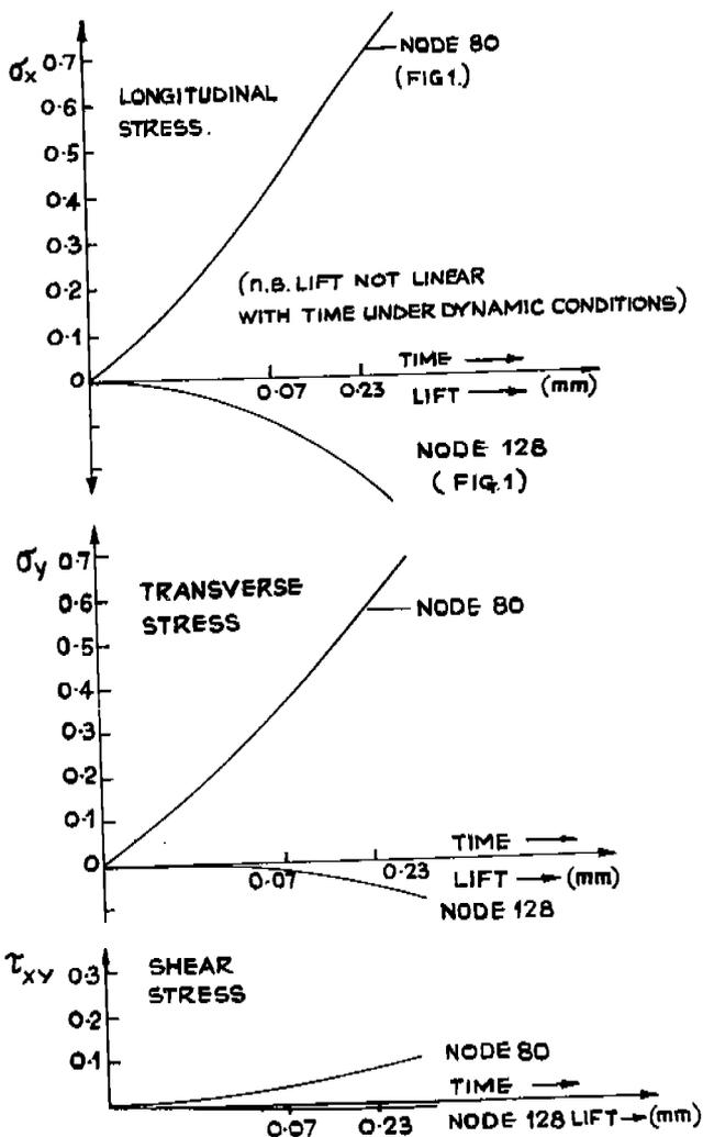
FIG.12. THEORETICAL STRESSES ( $N/mm^2$ ) VERSUS FREE LIFT FOR SUCTION VALVE REED
