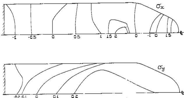
FIG. 3 STATIC FIELD STRESS (N/mm<sup>2</sup>) FOR HALF SUCTION VALVE REED AFTER TOUCHING THE STOP AT REED TIP. PRESSURE LOADING 2 bar.
