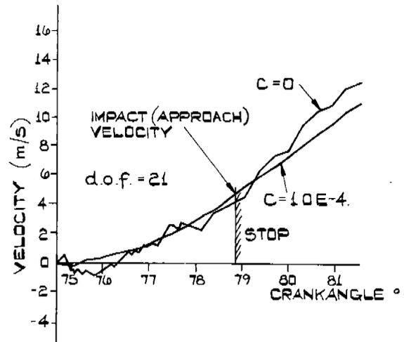
FIG. 10. SUCTION VALVE TIP VELOCITY
