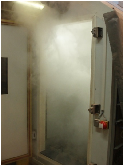
Fig. 1. Salt spray chamber with samples in position and door open during wet cycle.
