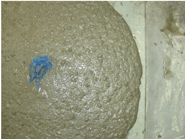
Fig. 3. OPC slump flow test concrete illustrating good cohesion in the mix
