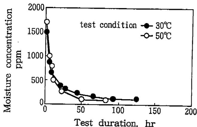
Fig.4 Change in moisture concentration with test duration.
