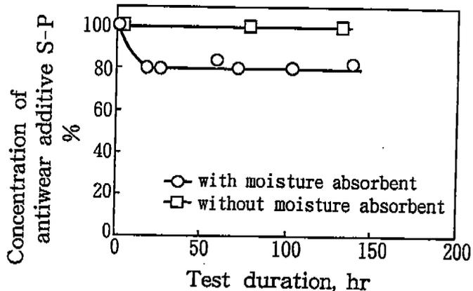
Fig.5 change in concentration of antiwear additive S - P
