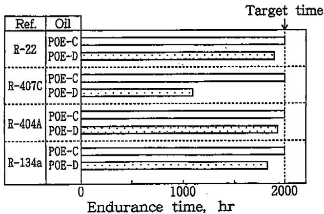
Fig.7 High load acceleration test duration of compressor
