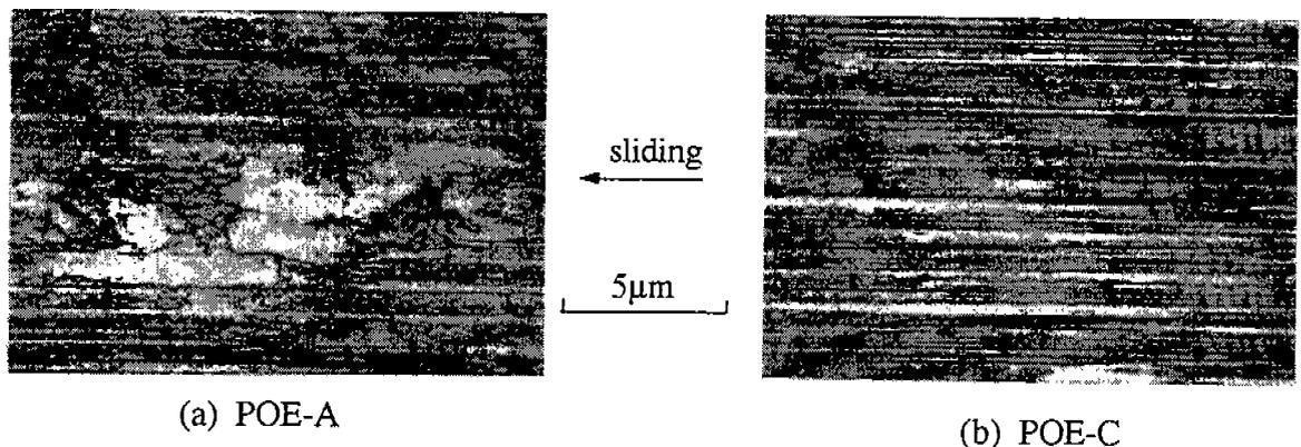
Fig.7 Sliding surfaces of rings after the test
