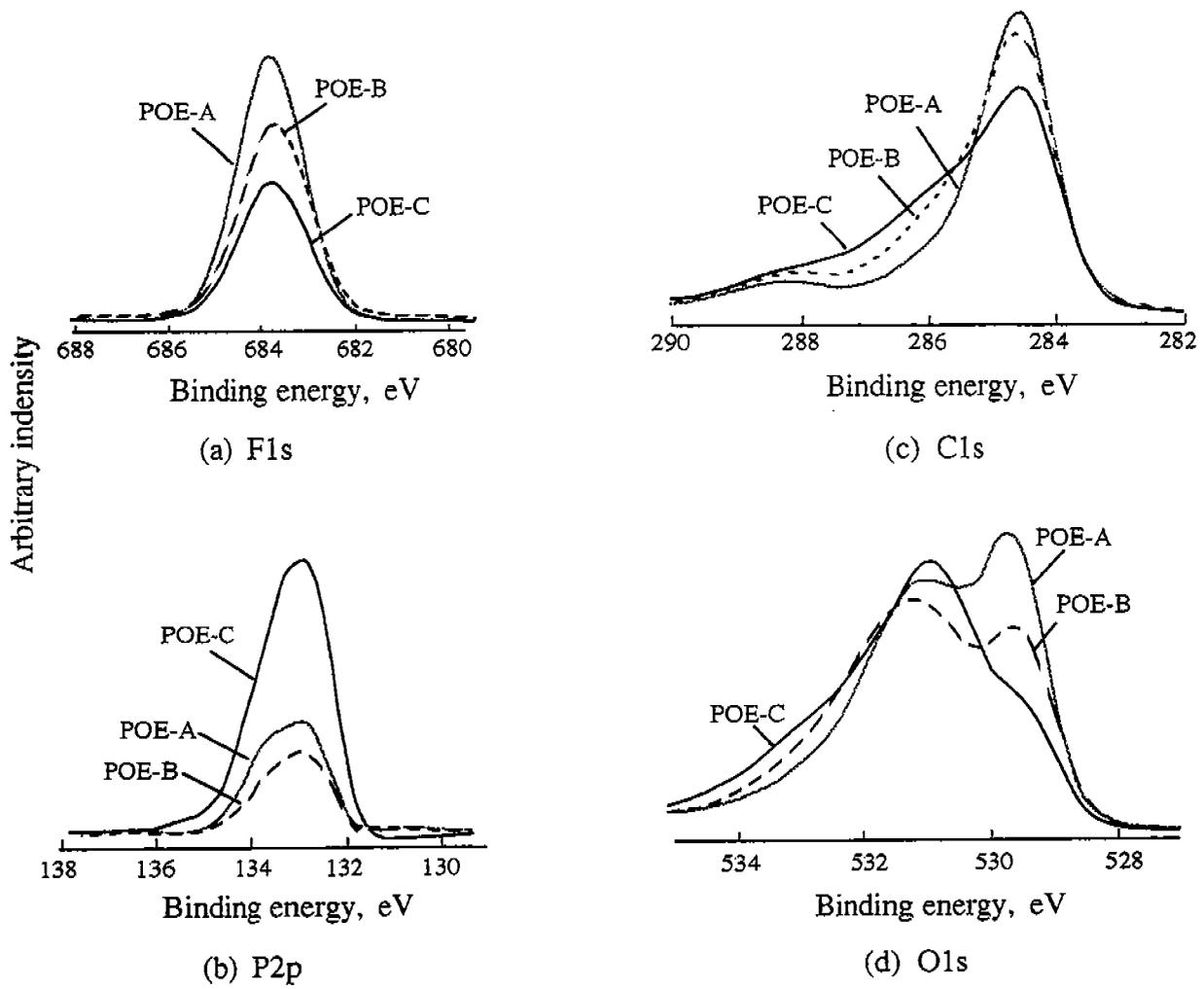
Fig.8 XPS spectra for sliding surfaces of rings with POEs
