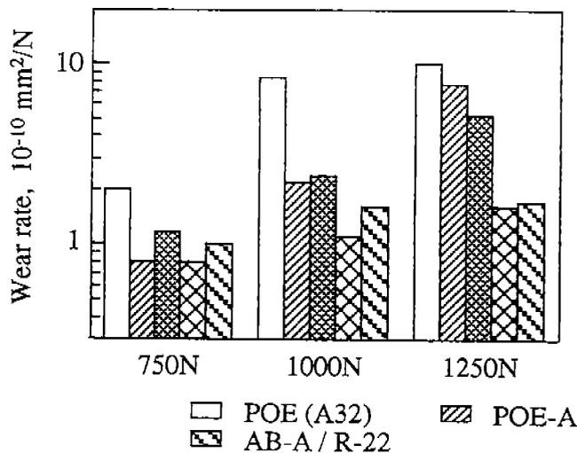
Fig.5 Wear rate for formulated oils vs load
