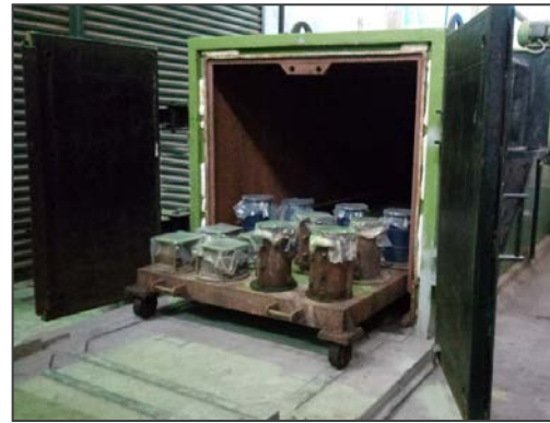
Fig. 2. Specimen in steam chamber curing
