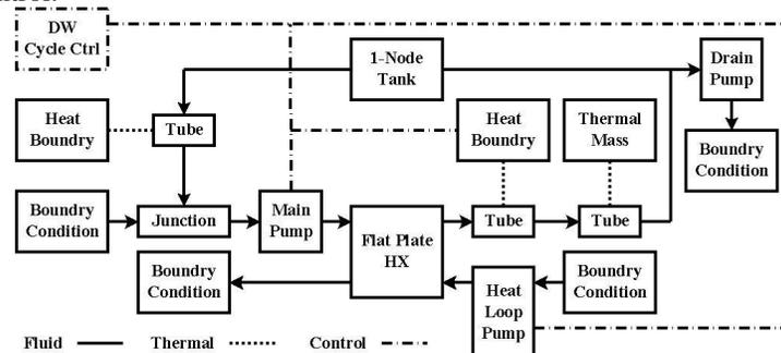
Figure 5: Dishwasher Modelica Model Diagram with Controller
