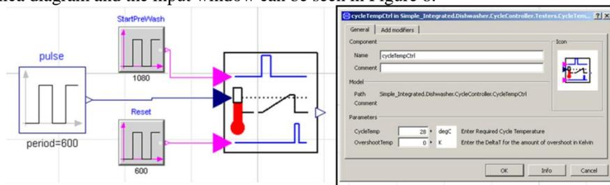
**Figure 8:** DW Modelica Diagram and Parameter Window for the Temperature Controller
