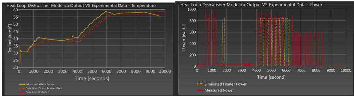
**Figure 12:** Heat Loop Driven DW Simulated Versus Experimental Data (Left) Temperatures – (Right) Electric Element Power
