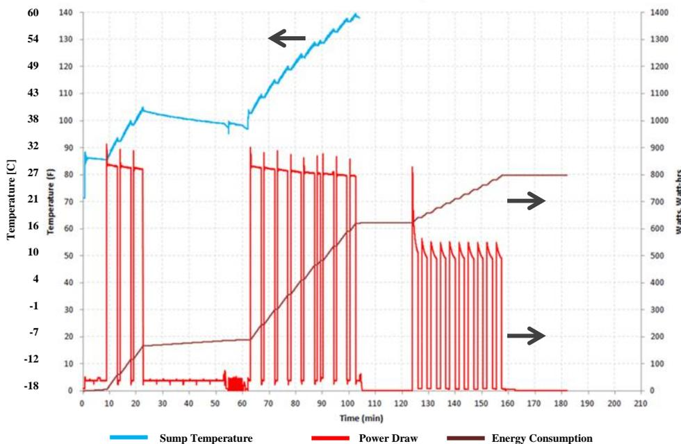
**Figure 2:** Example DW Sensing Wash Cycle with Sump Temperature, Power Consumption and Accumulated Energy (Whirlpool Corp., 2017)
