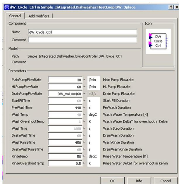
Figure 9: Parametric Inputs for DW Cycle Controller
