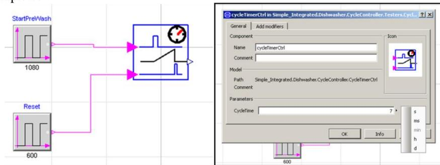
**Figure 7:** DW Modelica Diagram and Parameter Window for the Timer Controller
