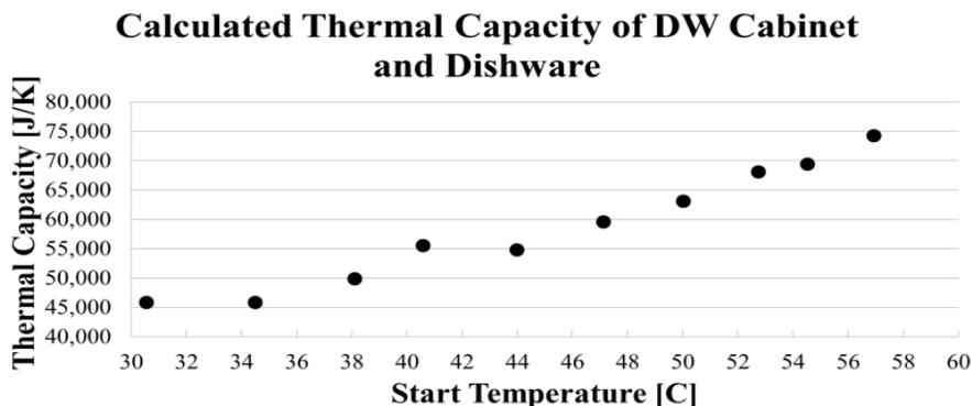
**Figure 3:** Calculated Thermal Capacity of Entire DW during Heating Cycles as Function of Starting Water Temperature
