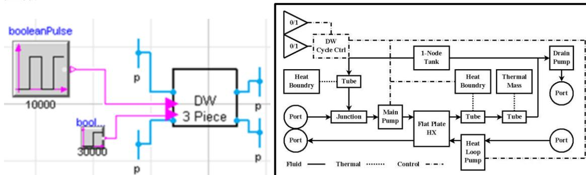
Figure 6: Boundary Conditions for DW Modelica Model
