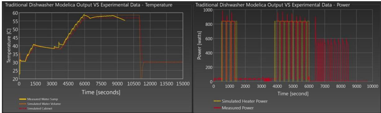
**Figure 10:** Traditional DW Operation Simulated Versus Experimental Data (Left) Temperatures - (Right) Electric Element Power
