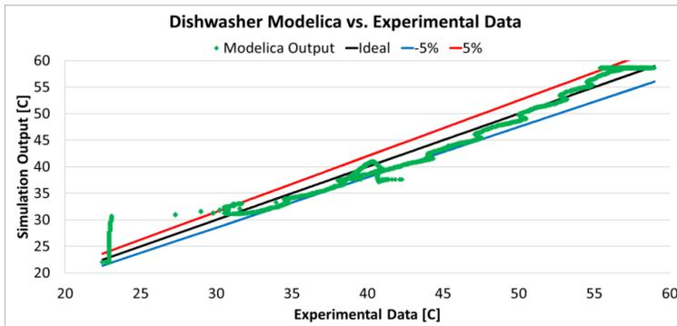
**Figure 11:** Water Sump Temperature – Simulated vs Experimental
