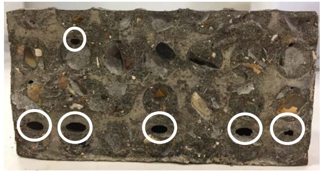
**Fig. 10.** Air voids at the spacer-concrete interface
