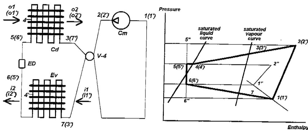
Figure 1. Air Conditioning System with Heat Pump.
