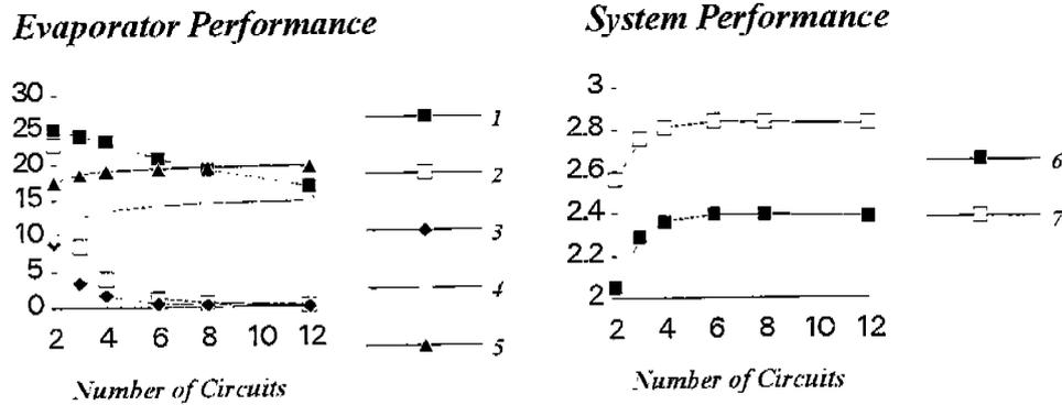
**Figure 3. Evaporator and system Performance on Number of Circuits.** 1 - Film Coefficient of Boiling Refrigerant,  $10 \cdot \frac{kW}{m^2 \cdot K}$ ; 2 - Refrigerant Pressure Drop, psi; 3 - Refrigerant Temperature Drop, K; 4 - Temperature Head at Refrigerant Inlet, K; 5 - Mean Logarithmic Temperature Difference, K; 6 - Cooling Capacity,  $10^{-4} \cdot Btuh$ ; 7 - COP.
