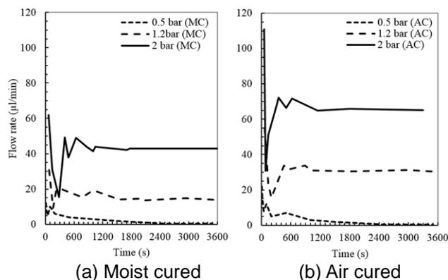
**Fig.5.** Air flow rates under different test pressure
