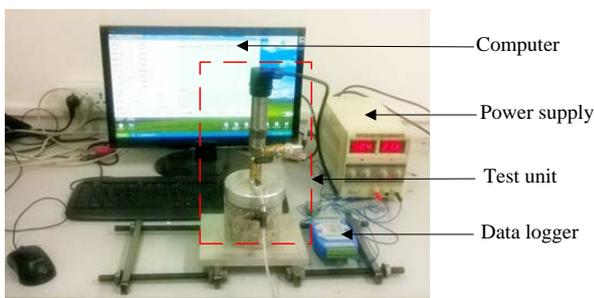
**Fig.4** Test set up of the new laboratory air permeability test device
