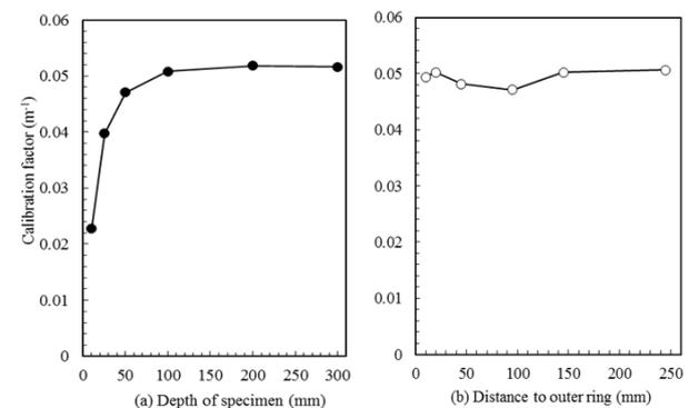
**Fig.3.** Calibration factor under different specimen depths and distances to outer side of the seal
