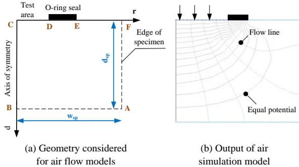
**Fig.2** Configuration of flow models to study influence of configuration on calibration factor
