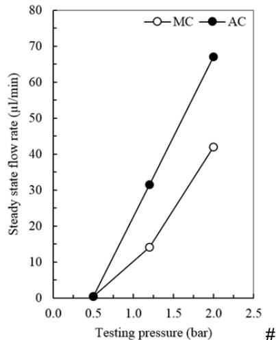
**Fig. 6.** Relationship between test pressure and steady state air flow rate (The air flow rates at different pressure was converted to the flow rates at 1 atm)
