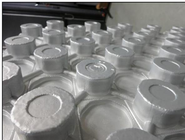
**Figure 3:** Cylindrical insulation foam matrix
