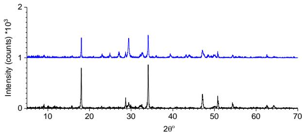
**Fig. 2.** XRD of cement paste made with OPC, exposed to 0% and 7% CO<sub>2</sub>
