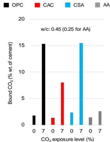
**Fig. 6.** Bound CO<sub>2</sub> levels in cement paste made with OPC and ACMs, exposed to 0% and 7% CO<sub>2</sub>
