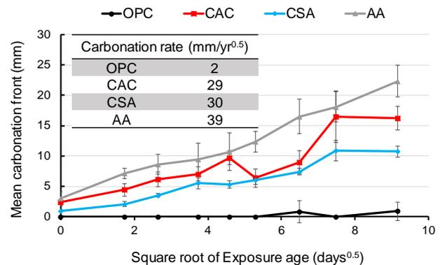
**Fig. 8.** Mean carbonation front of concrete samples made with OPC and ACMs, exposed to 7% CO<sub>2</sub>, at different exposure ages
