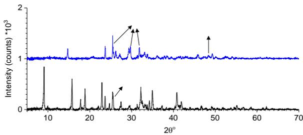
**Fig. 4.** XRD of cement paste made with CSA, exposed to 0% and 7% CO<sub>2</sub>
