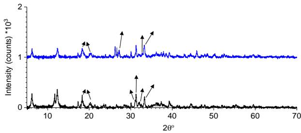
**Fig. 3.** XRD of cement paste made with CAC, exposed to 0% and 7% CO<sub>2</sub>
