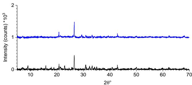
**Fig. 5.** XRD of cement paste made with AA, exposed to 0% and 7% CO<sub>2</sub>
