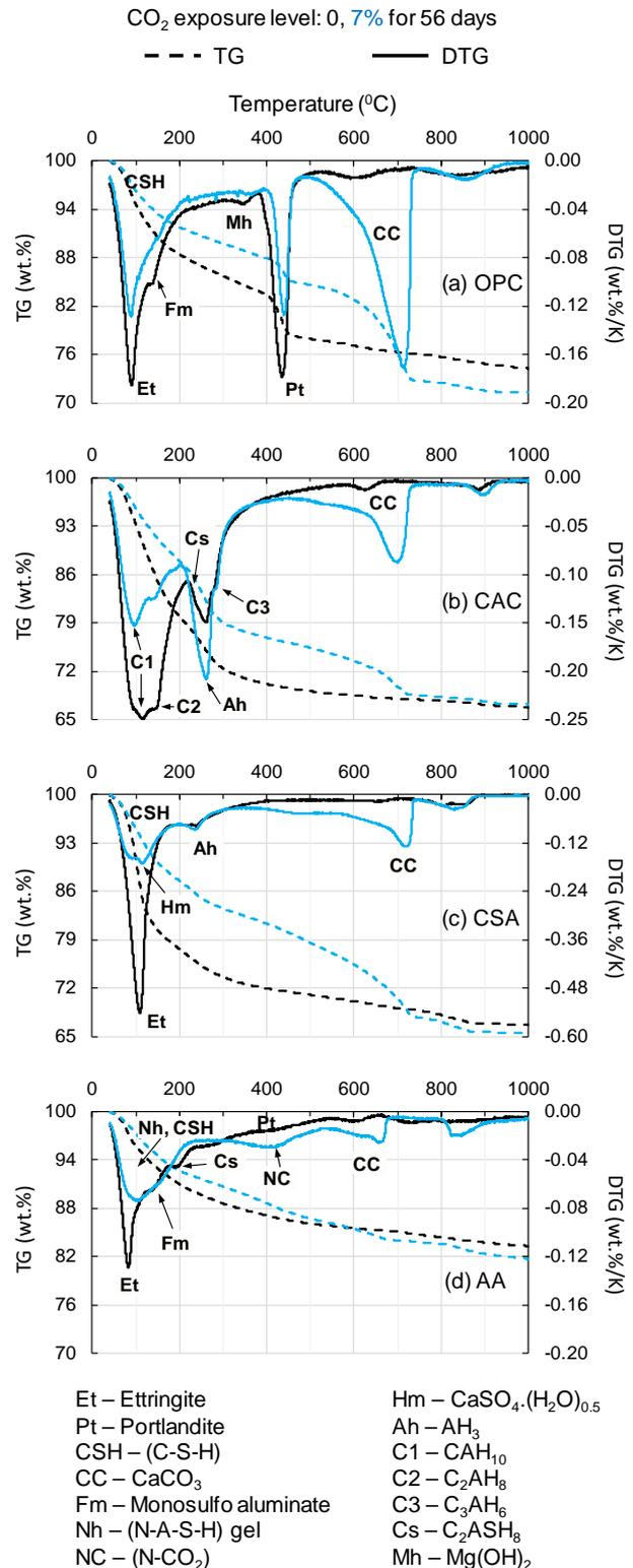
**Fig. 1.** TG and DTG curves of cement pastes made with (a) OPC, (b) CAC, (c) CSA, and (d) AA; exposed to 0% and 7% CO<sub>2</sub>
