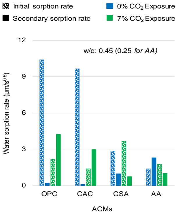
**Fig. 7.** Initial and secondary sorption rate of cement mortar samples made with OPC and ACMs, exposed to 0% and 7% CO<sub>2</sub>
