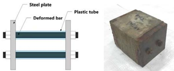
**Fig. 1.** Specimen for confined compressive strength test
