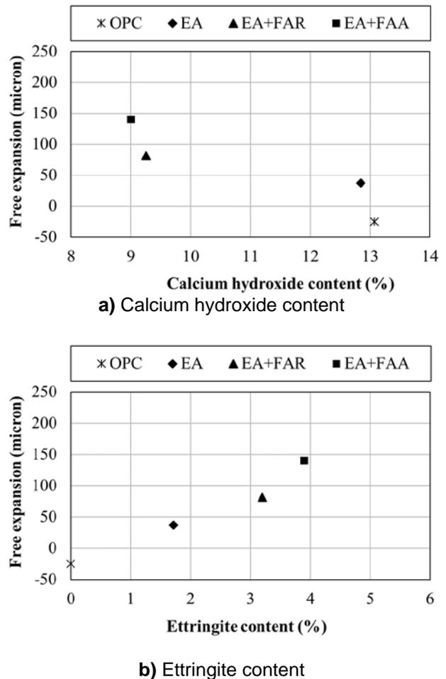
**Fig. 6.** Relationship between results of expansive products derived from XRD analysis and free expansion of concrete containing different types of fly ash at the age of 7 days
