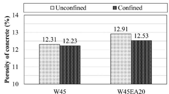
**Fig. 9.** Porosity of concrete made under unconfined and confined conditions at the age of 7 days
