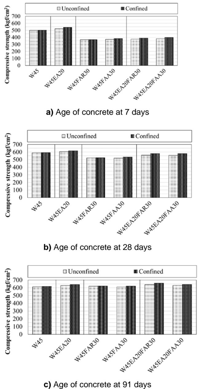
**Fig. 8.** Unconfined and confined compressive strengths of concrete containing different types of fly ash
