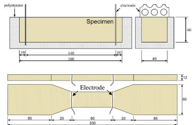
**Fig. 2.** Dimensions of prismatic specimen for hydration study and dog-bone shaped specimen for piezo-impedance study. All dimensions in mm
