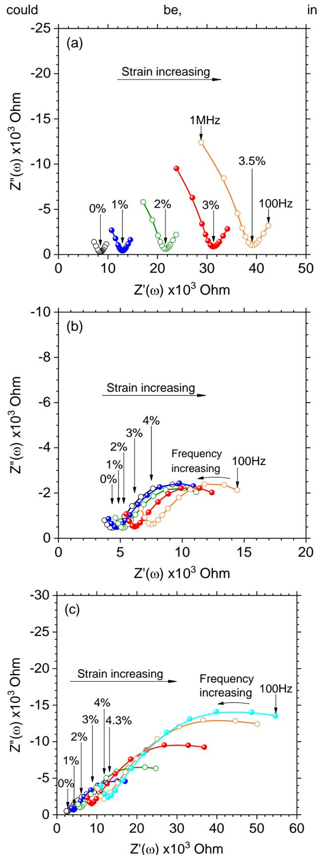
**Fig. 5.** Piezo-impedance response: (a) ECC; (b) ECC+CS and (c) ECC+CS+MCF1%
