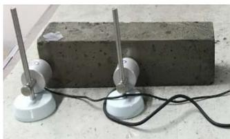
Fig. 2. Fundamental transverse frequency test
