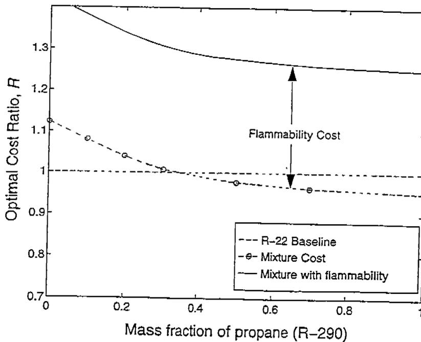
Figure 2: Optimal system cost ratio for R-227EA/R-290 mixtures with HCFC-22 as the baseline refrigerant
