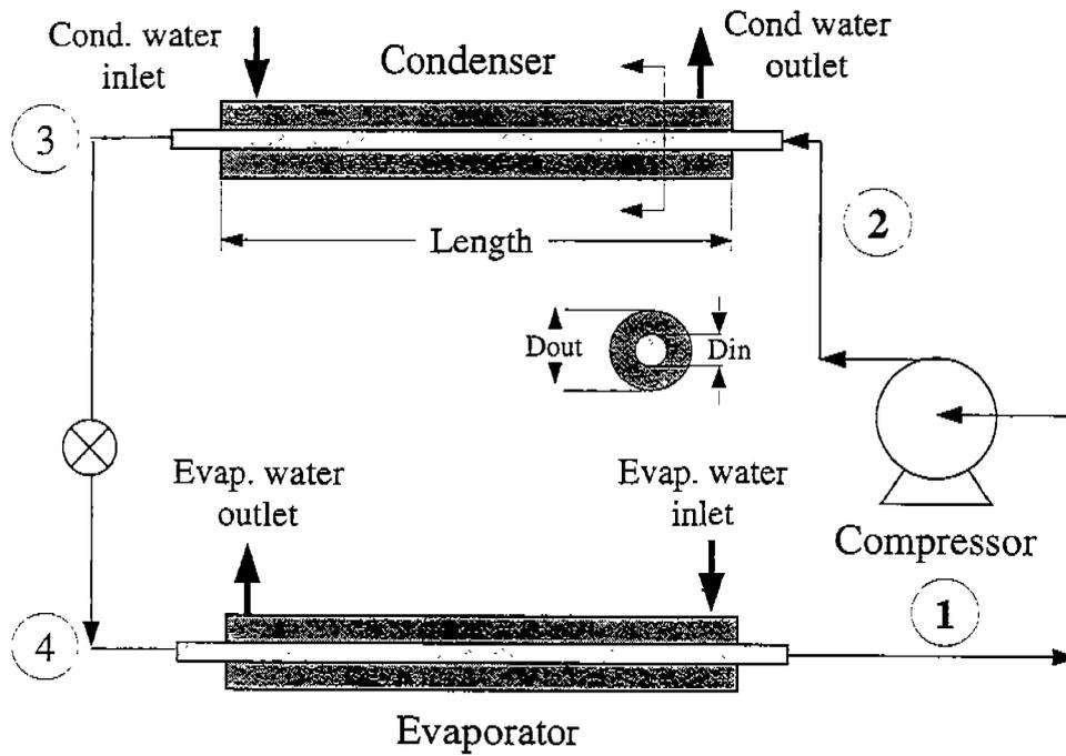
Figure 1: Schematic of the simplified system
