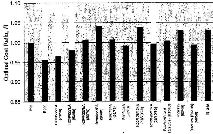
Figure 3: Optimal system cost ratios for various refrigerants with R-22 as the baseline
