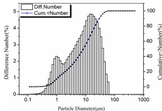
Fig. 2. The particle size distribution of slag
