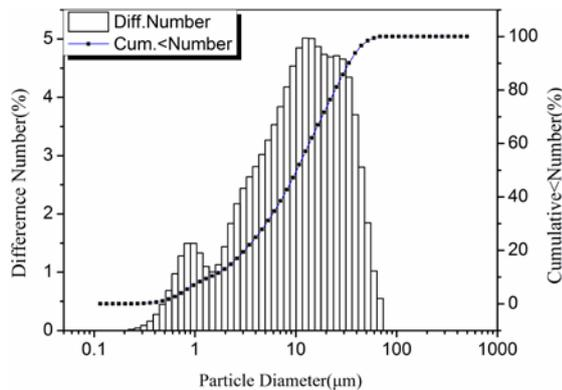
Fig. 1. The particle size distribution of cement
