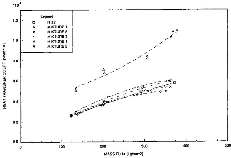
**Figure 2 Heat Transfer Comparison at -2°C Based on Mass Flux**
