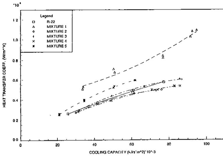
**Figure 3 Heat Transfer Comparison at 4°C Based on Mass Flux**
