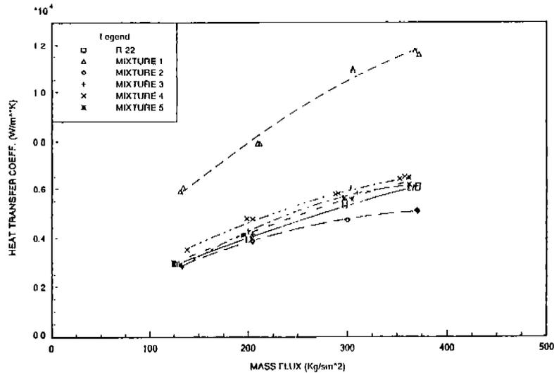
**Figure 4 Heat Transfer Comparison at -2°C Based on Cooling Capacity**
