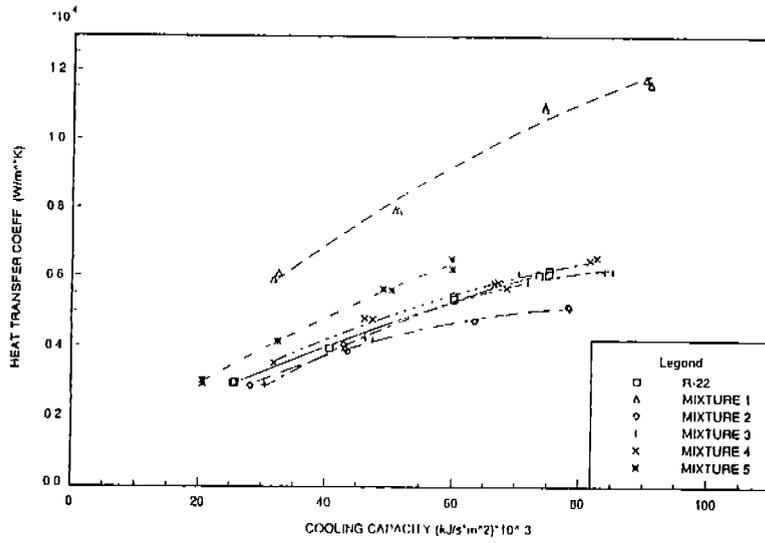
**Figure 5 Heat Transfer Comparison at 4°C Based on Cooling Capacity**
