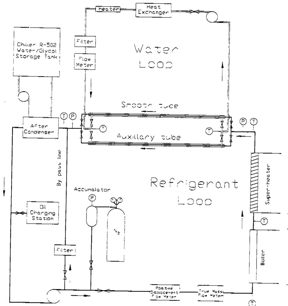
**Figure 1 Schematic of In-Tube Test Facility**
