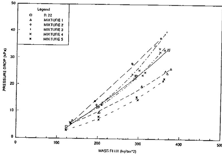
**Figure 6 Pressure Drop Comparison at -2°C**
