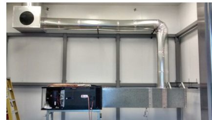
■ Variable speed heat pump in the psychrometric test chamber.
