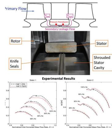
The schematic model of the experimental setup demonstrates the flow path of secondary leakage flows and the placement of the pressure transducers across the knife seals in the shrouded stator cavity. From conservation of momentum, the change in pressure ( $\Delta p$ ) across the knife seals can be used to quantify the secondary leakage flow through the shrouded stator cavities, providing boundary conditions for a CFD mesh at various operating conditions.
