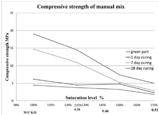
**Fig. 7.** Compressive strength of manual mix cementitious materials
