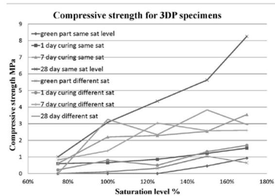
**Fig. 6.** Compressive strength of 3DP parts without a heating cure.
