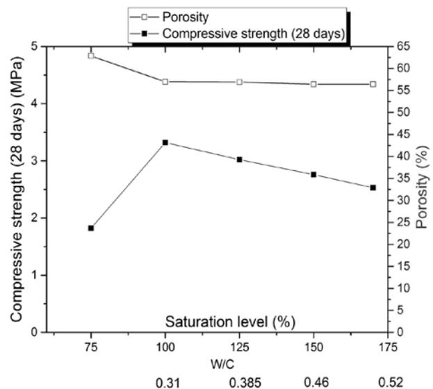
**Fig. 17.** Schematic illustration of porosity vs. compressive strength
