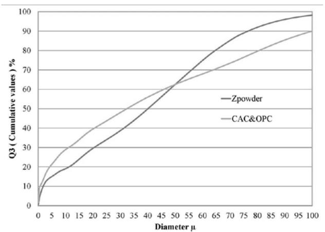
**Fig. 5.** Particle size distributions for the powders
