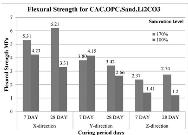
**Fig. 10.** Flexural strength of cementitious prism in different directions (X, Y, and Z) and saturation levels for 170% and 100% saturation levels
