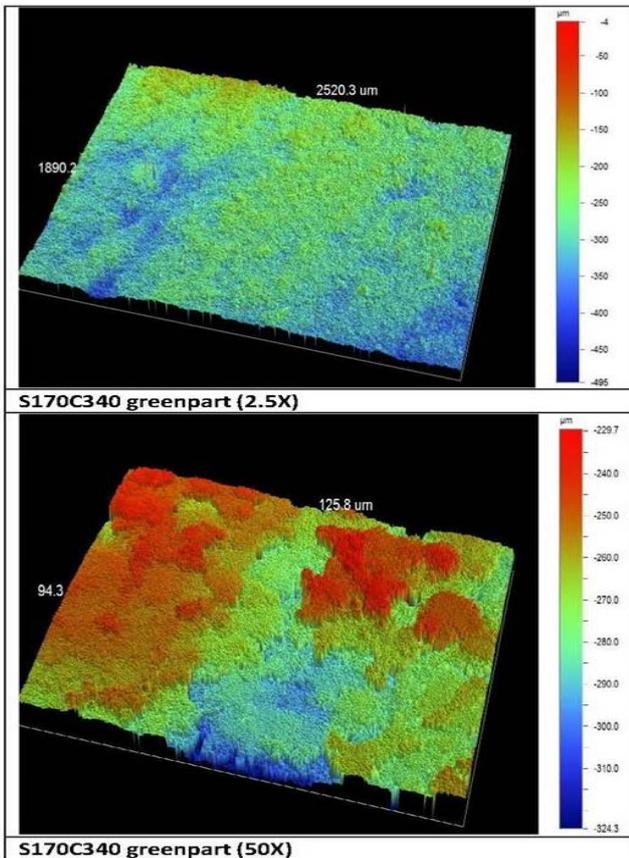
**Fig. 14.** Some 3D profiling image for 3D printed samples (green part)
