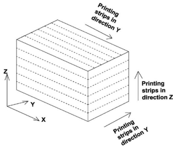
**Fig. 3.** Directional depiction of the 3D printing process.
