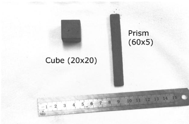
**Fig. 13.** Printed cube and prism via inkjet printer (3D Zprinter @150) (dimensions are in mm)
