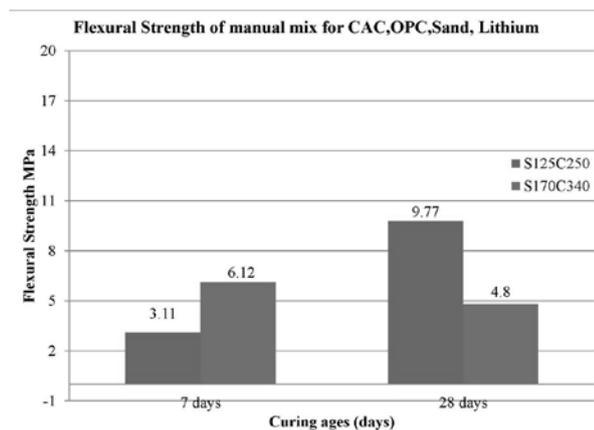
**Fig. 11.** Flexural strength for manual mortar mix materials for saturation levels S125C250& S170C340
