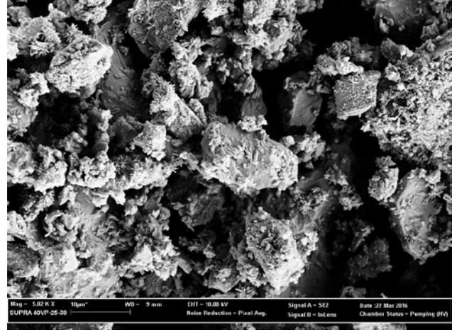
**Fig. 12.** SEM image of 3D printed samples, (10 µm).
