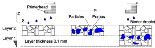
**Fig. 1.** Layer explanation and powder/binder interaction between layers
