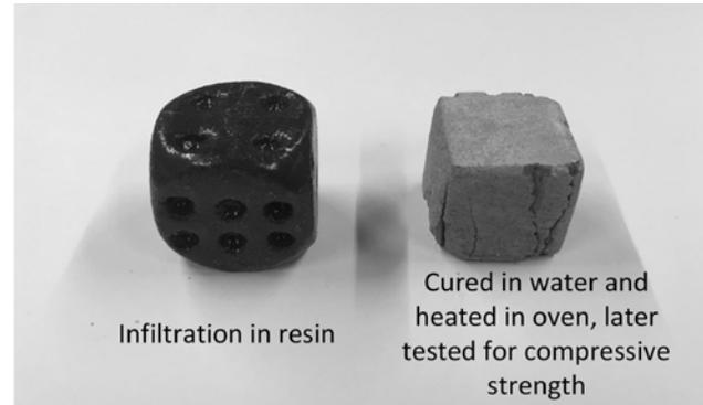
**Fig. 16.** 3DP specimens are cured by different agents
