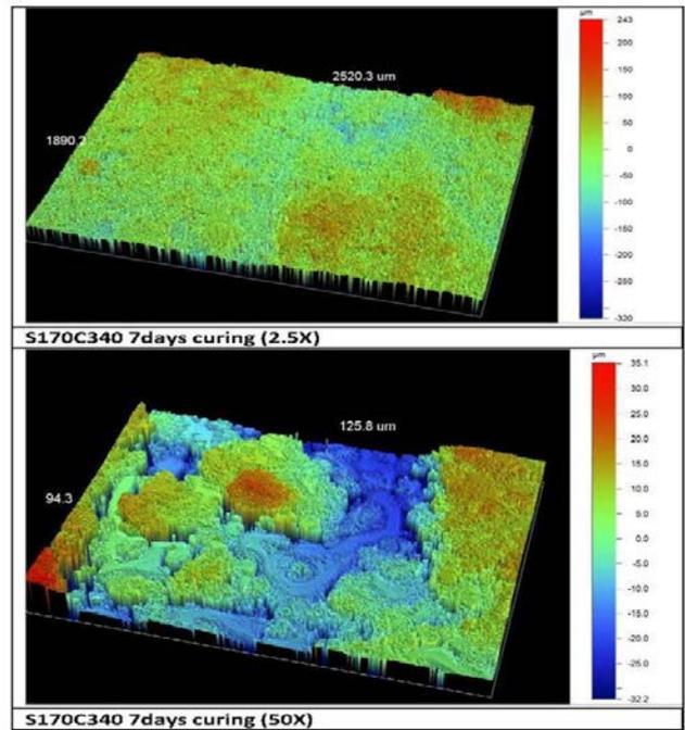
**Fig. 15.** Some 3D profiling image for 3D printed samples (after 7days curing).
