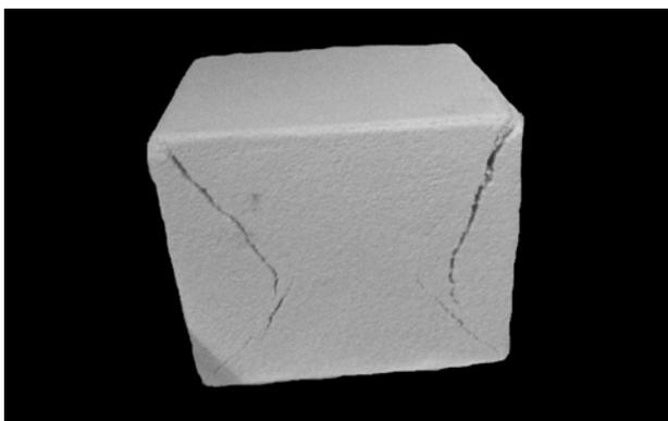
**Fig. 8.** Diagonal crack inside the Z-powder specimen (50x50) mm.
