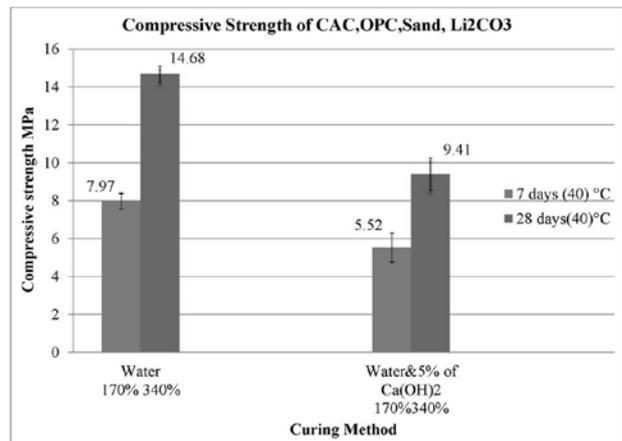
**Fig. 9.** Compressive strength of mortar mix 3DP materials after dried in an oven for S170C340
