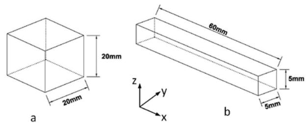
**Fig. 2.** (a) cubic specimens (20×20×20mm), (b) prism specimens (60×5×5mm).
