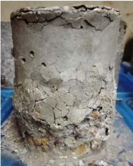
**Fig. 10.** Map cracking and detachment of a surface layer from silane treated concrete cylinders
