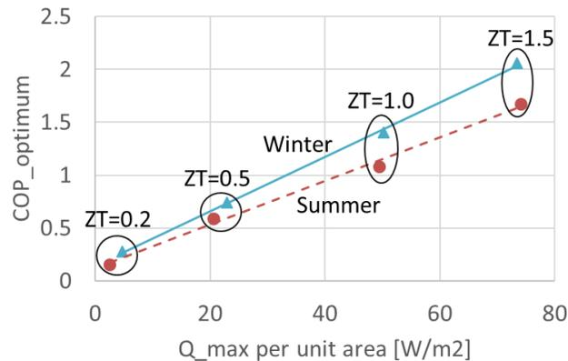
Figure 10. Heat pump performance map COP vs  $Q_{\max}$  of ZT value dependence.
