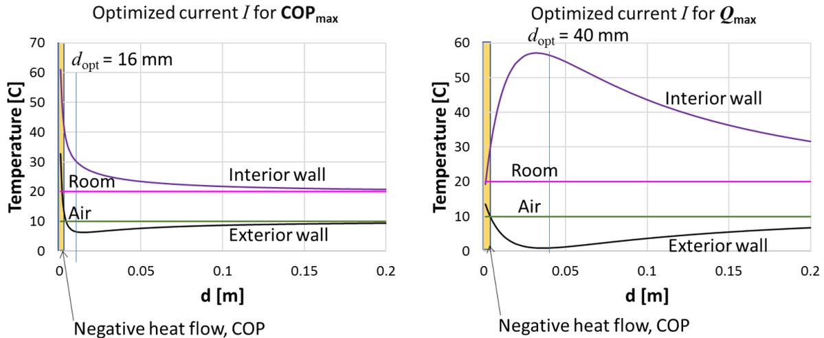
**Figure 8:** Temperatures vs leg length  $d$  with optimizing current  $I$  for COP or  $Q_{max}$ . Condition is the same as Fig. 7.
