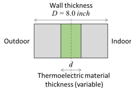
**Figure 2:** Cross section of the thermoelectric embedded wall. The wall consists of thermoelectric material (thickness of  $d$ ,  $D \geq d \geq 0$ ) with electrical contacts at the center and concrete portion on both side.
