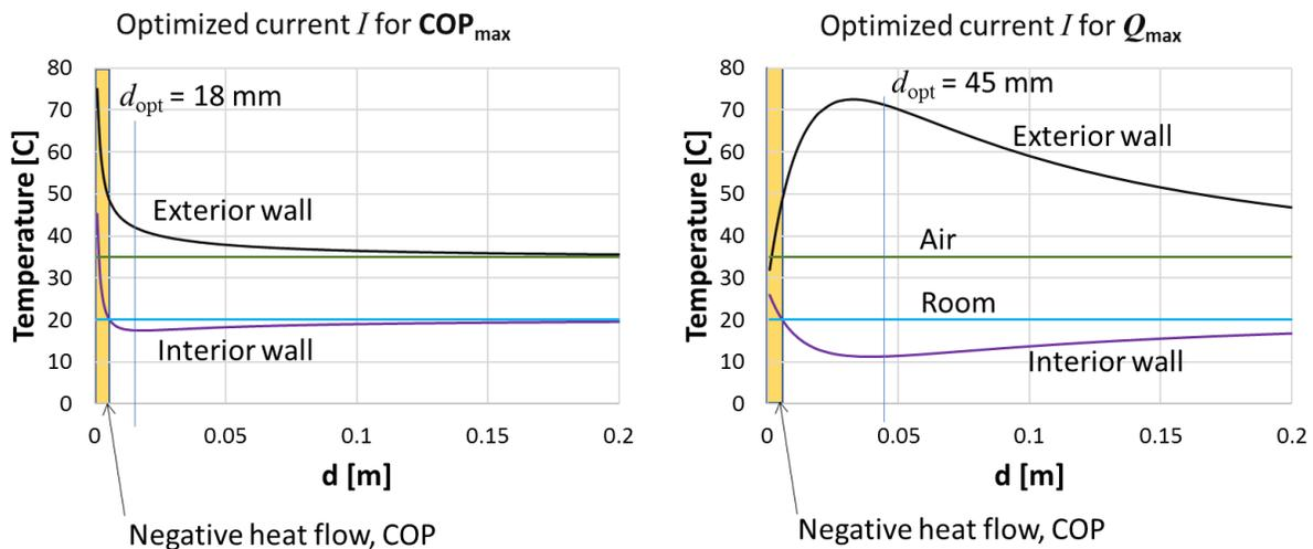
**Figure 6:** Temperatures vs leg length  $d$  with optimizing current  $I$  for COP or  $Q_{\max}$ . Condition is the same as Fig.5.
