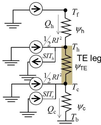
**Figure 1:** Thermal network model of thermoelectric heat pump. The heat flows related to current  $I$  is the heat generation or removal by Joule effect and Peltier effect at the terminals of the thermoelectric leg.
