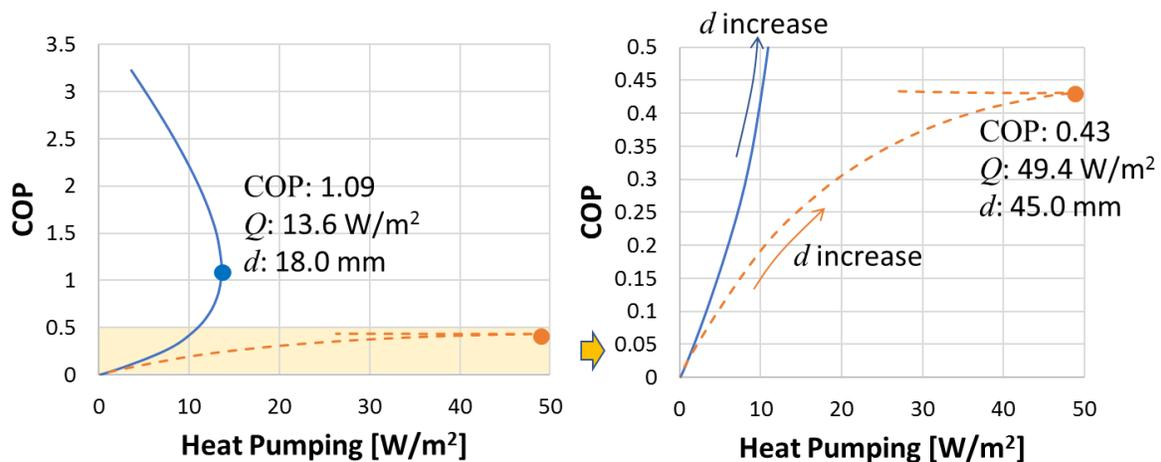
**Figure 5:** COP vs Heat pumping. Condition: Summer 35 °C outdoor and 20 °C room. Thermoelectric  $Z = 2.82 \times 10^{-3}$  [1/K] ( $ZT \sim 0.87$ ) and fill factor  $F = 4\%$  with cross section of leg 2 mm x 2 mm. Right hand side is zoom up.
