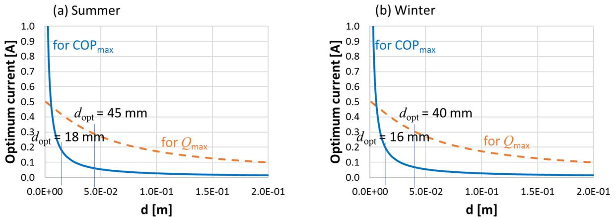
**Figure 9:** Relation between the optimum current  $I$  and optimum leg length  $d$  (a) Summer and (b) winter.
