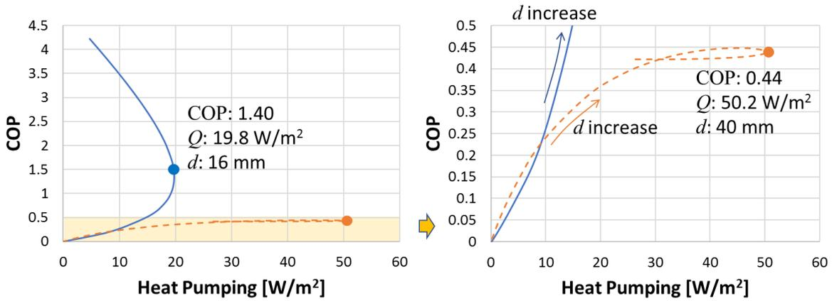
**Figure 7:** COP vs Heat pumping. Condition: Windy winter day 10 °C outdoor air and 20 °C room. Thermoelectric  $Z = 2.82 \times 10^{-3} [1/K]$  ( $ZT \sim 0.87$ ) and fill factor  $F = 4\%$  with cross section of leg 2 mm x 2 mm.
