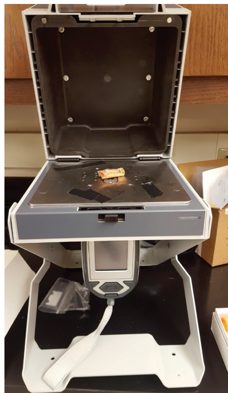
Sample condor bone fragment is placed in a portable L-shell x-ray fluorescence device.
